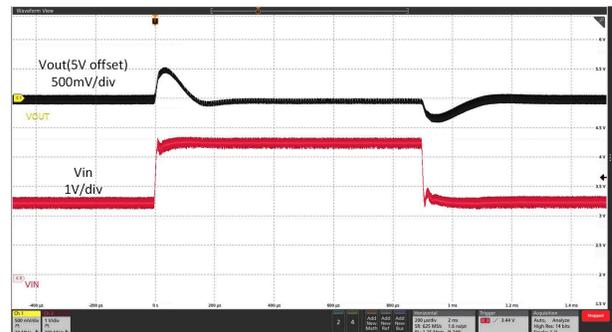
$V_{IN} = 2.5\text{ V}$  to  $4.6\text{ V}$  with 20- $\mu\text{s}$  slew rate,  $V_{OUT} = 5\text{ V}$ ,  $I_{OUT} = 800\text{ mA}$
