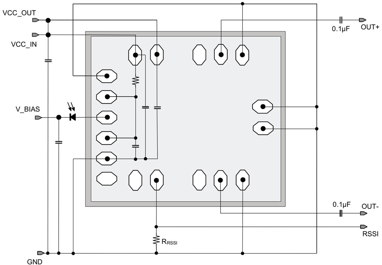
Figure 16. Basic Application Circuit for APD Receivers
