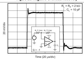
Figure 29. Small-Signal Step Response (100 mV)
