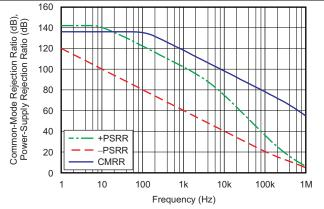
Figure 12. CMRR and PSRR vs Frequency
