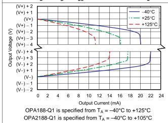
Figure 11. Output Voltage Swing vs
