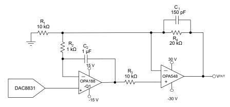
Figure 48. Programmable Power Supply
