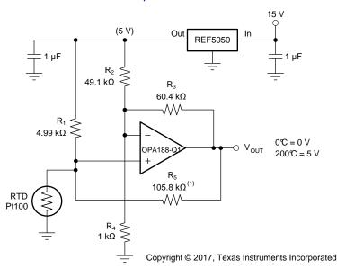
(1) R<sub>5</sub> provides positive-varying excitation to linearize output.
