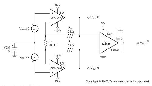
(1)  $V_{OUT} = V_{DIFF} \times (41 / 5) + (Ref 1) / 2$ .
