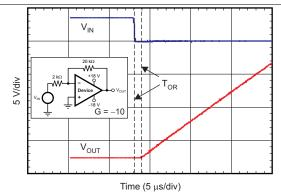
Figure 27. Positive Overload Recovery
