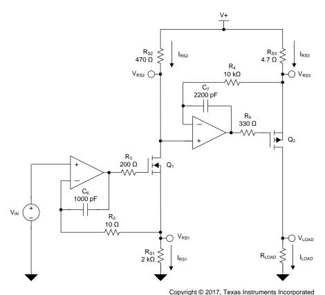
Figure 43. High-Side Voltage-to-Current (V-I) Converter
