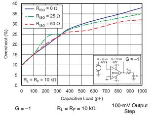
Figure 41. Small-Signal Overshoot Versus Capacitive Load
