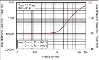
Figure 18. THD+N Ratio vs Frequency
