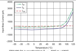
OPA188-Q1 is specified from  $T_A = -40$ °C to +125°C OPA2188-Q1 is specified from  $T_A = -40$ °C to +105°C
