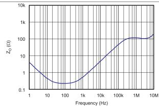
Figure 23. Open-Loop Output Impedance vs Frequency
