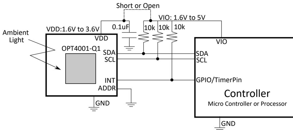
Figure 6-1. Functional Block Diagram of the OPT4001-Q1
