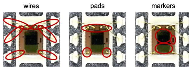
**Figure 8-5. Identification Features for Pin 1 on the Package**
