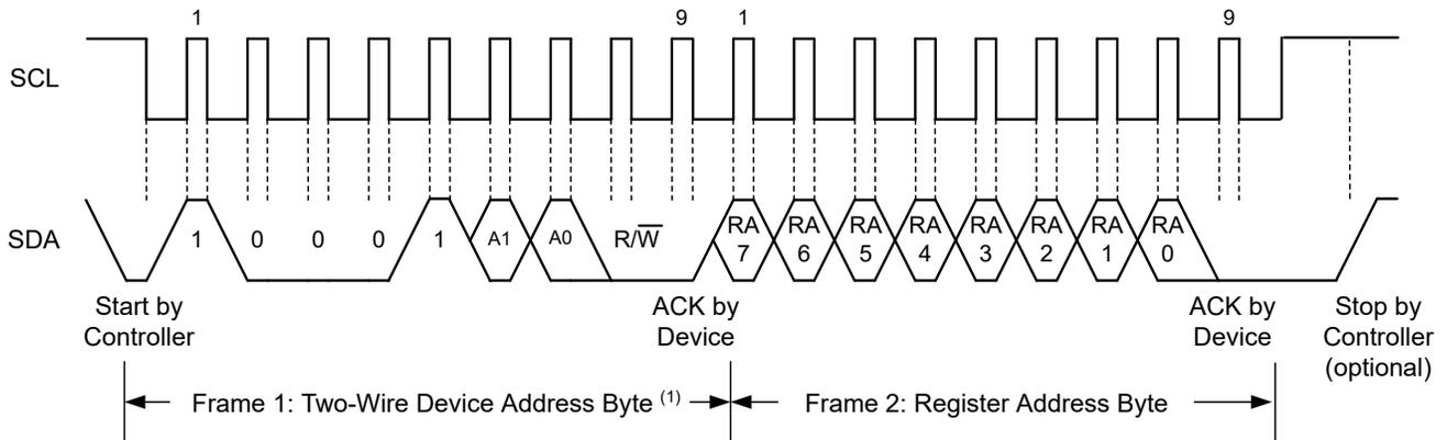
**Figure 6-5. Setting the I<sup>2</sup>C Register Address**
