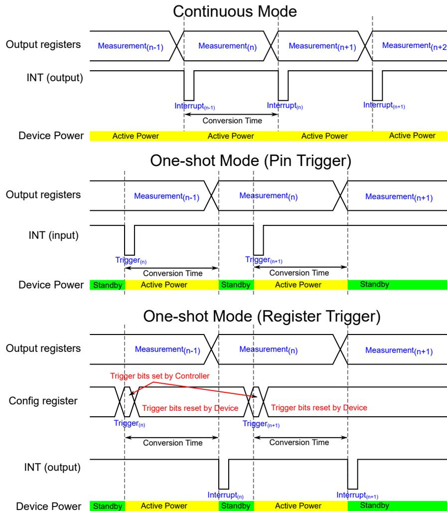
**Figure 6-3. Timing Diagrams for Different Operating Modes**
