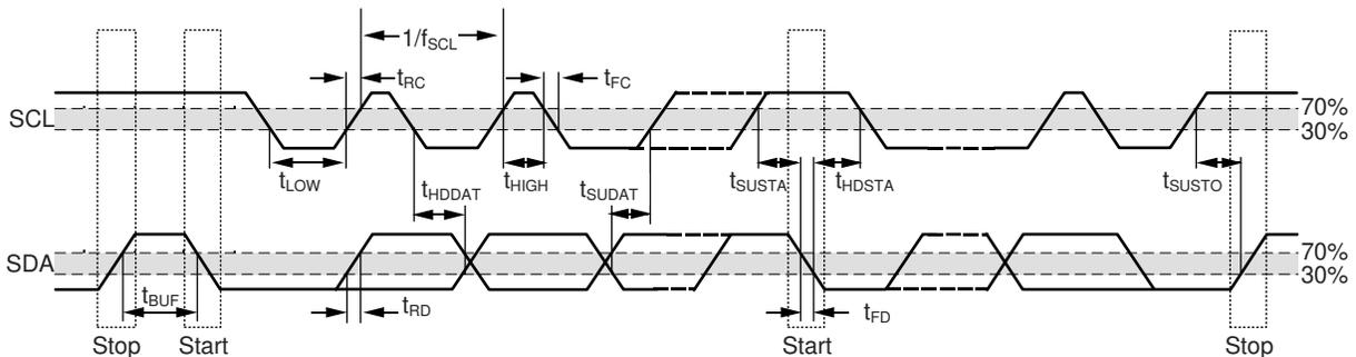
**Figure 5-1. I<sup>2</sup>C Detailed Timing Diagram**
