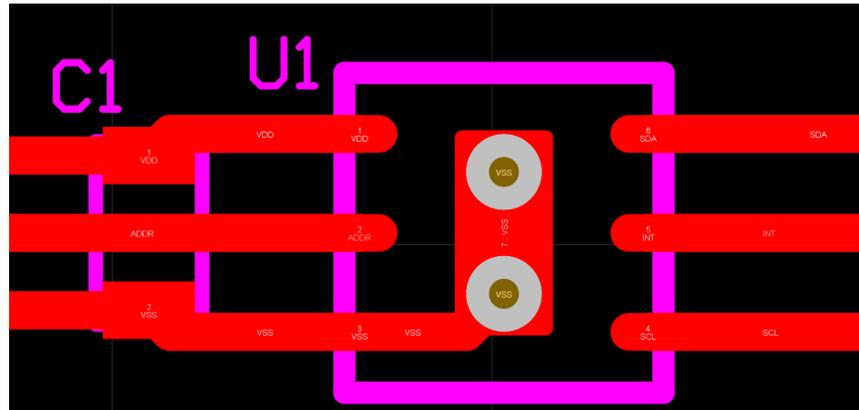
**Figure 8-6. Layout Example for DNP Package**
