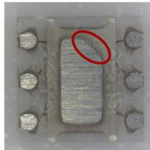
NOTE: The bottom side of the device features an angled feature to denote pin 1.
