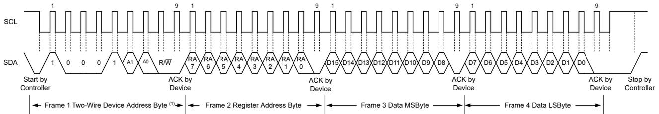
**Figure 6-6. I<sup>2</sup>C Write Example**
