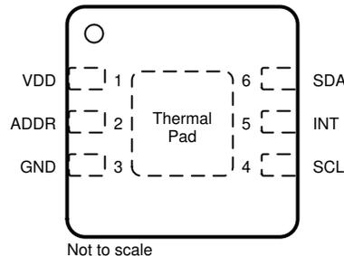
**Figure 4-1. DNP Package, 6-Pin USON
