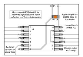
Figure 8-4. Layout Diagram
