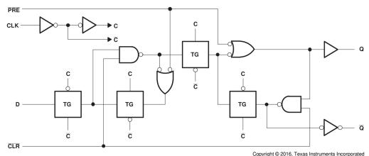
Logic Diagram, Each Flip-Flop (Positive Logic)
