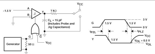
Generators: PRR = 1 MHz, 50% Duty Cycle, tr <6 ns, Z\_0 = 50  $\Omega$
