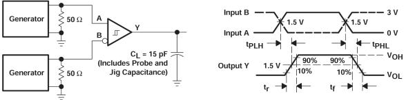
Generators: PRR = 1 MHz, 50% Duty Cycle,  $t_{r}$  <6 ns, Z\_{0} = 50  $\Omega$
