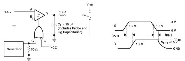
Generators: PRR = 1 MHz, 50% Duty Cycle,  $t_r < 6 \text{ ns}$ ,  $Z_0 = 50 \Omega$
