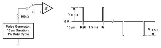
Figure 6-5. Test Circuit and Waveform, Transient Over-Voltage Test
