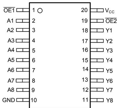
**Figure 4-1. DGS or PW Package,
