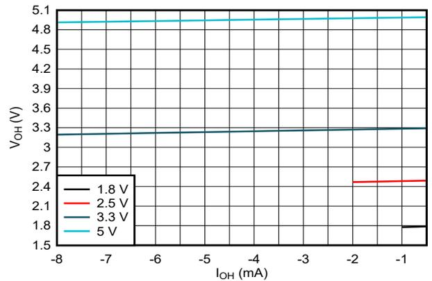
Figure 5-4. Output Voltage vs Current in HIGH State
