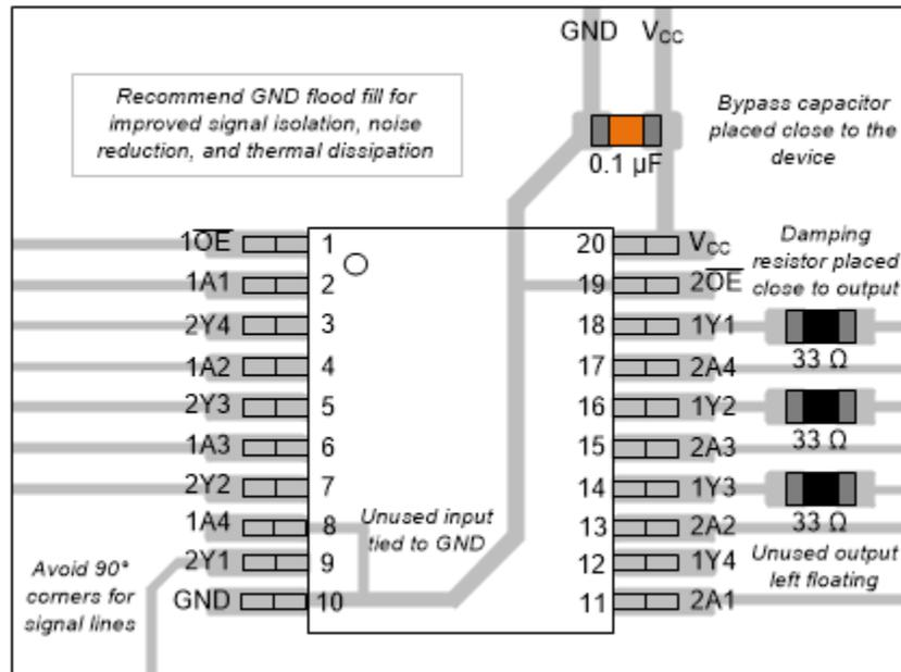
Figure 9-1. Layout Diagram
