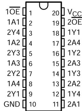
Figure 5-1. DW or PW Package (Top View)
