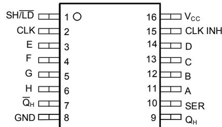
Figure 5-1. SN74HC165B-EP: PW Package, 16-Pin TSSOP (Top View)
