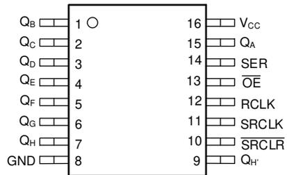
**Figure 5-1. SN74LV595B-EP: PW Package, 16-Pin TSSOP (Top View)**
