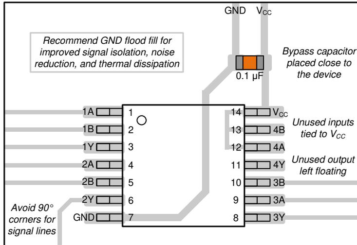
**Figure 10-1. Example Layout for the SN74LV6T17-EP**
