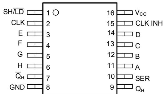
**Figure 4-1. PW Package, 16-Pin TSSOP (Top View)**
