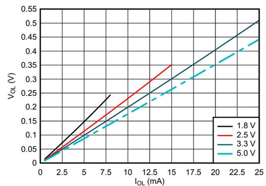
Figure 5-4. Output Voltage vs Current in LOW State
