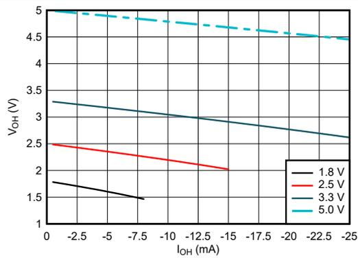
Figure 5-3. Output Voltage vs Current in HIGH State
