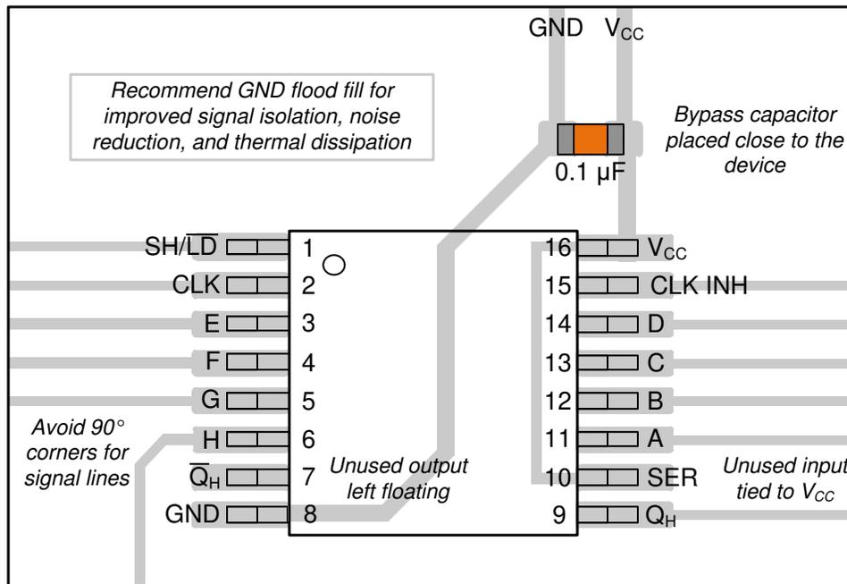
Figure 8-3. Example Layout for the SN74LV8T165 in TSSOP
