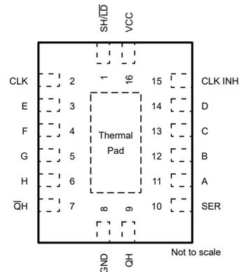
**Figure 4-2. BQB Package, 16-Pin WQFN (Top View)**
