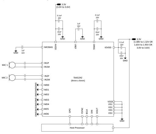
Figure 9-1. Stereo MEMS Microphone Block Diagram
