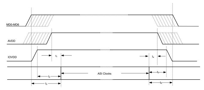
Figure 10-1. Power-Supply Sequencing Requirement Timing Diagram
