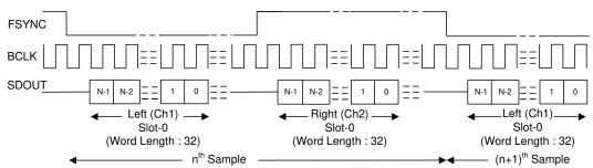
Figure 8-4. I<sup>2</sup>S Mode Protocol Timing (MD0 shorted to ground) in Target Mode
