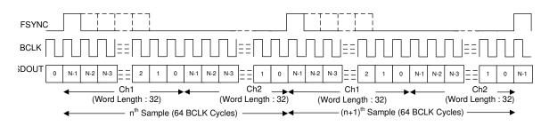
Figure 8-3. TDM Mode Protocol Timing (MD0 shorted to AVDD with 4.7K Ohms) In Controller Mode
