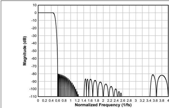
**Figure 6-21. Linear Phase Decimation Filter Magnitude Response**
