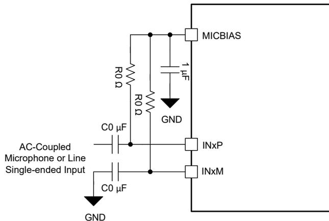
Figure 6-17. AC-Coupled Microphone or Line Single-Ended Input Connection
