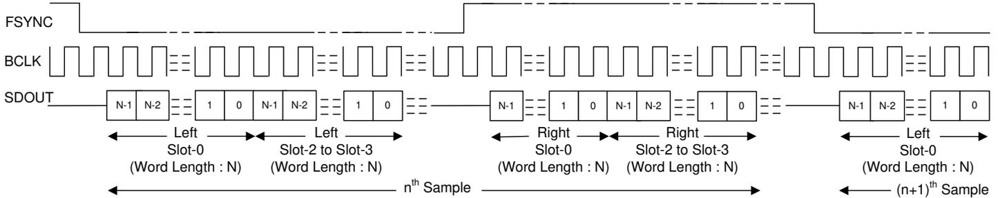
Figure 6-5. I<sup>2</sup>S Mode Standard Protocol Timing (PASI\_TX\_OFFSET = 0)
