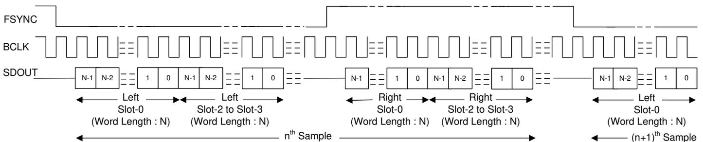
Figure 6-8. I<sup>2</sup>S Protocol Timing (PASI\_TX\_OFFSET = 0 and PASI\_BCLK\_POL = 1)
