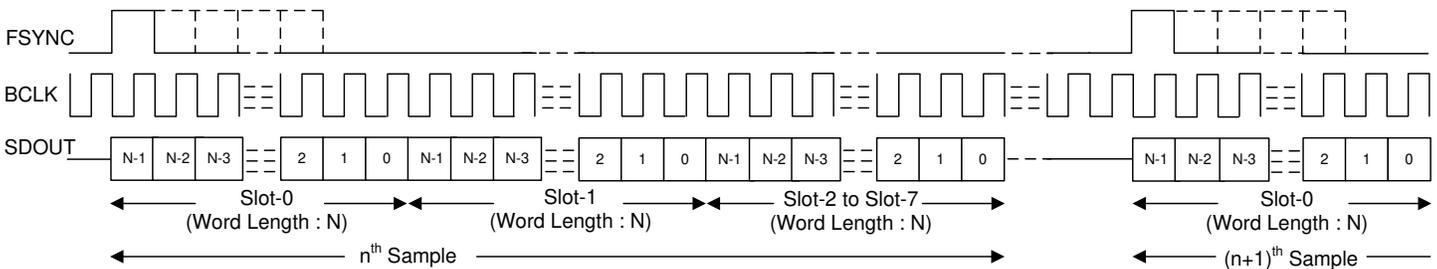
**Figure 6-4. TDM Mode Protocol Timing (PASI\_TX\_OFFSET = 0 and PASI\_BCLK\_POL = 1)**
