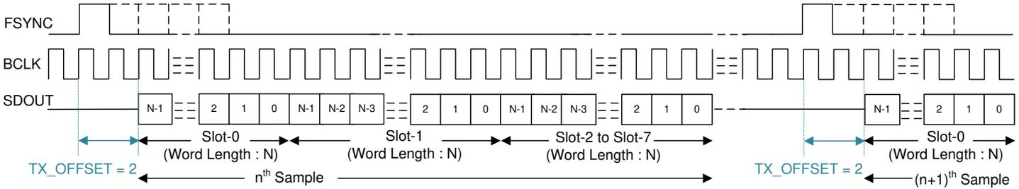
**Figure 6-2. TDM Mode Protocol Timing (PASI\_TX\_OFFSET = 2)**
