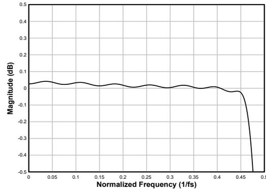
**Figure 6-22. Linear Phase Decimation Filter Pass-Band Ripple**
