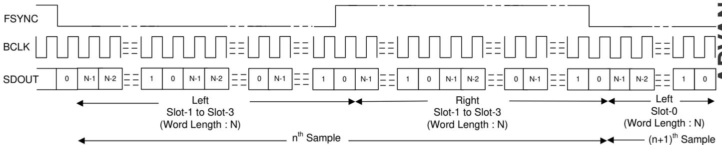
Figure 6-7. I<sup>2</sup>S Protocol Timing (No Idle BCLK Cycles, PASI\_TX\_OFFSET = 0)
