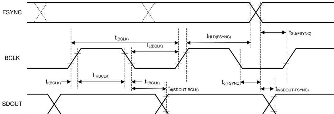
Figure 5-3. TDM, I<sup>2</sup>S, LJ Interface Timing Diagram
