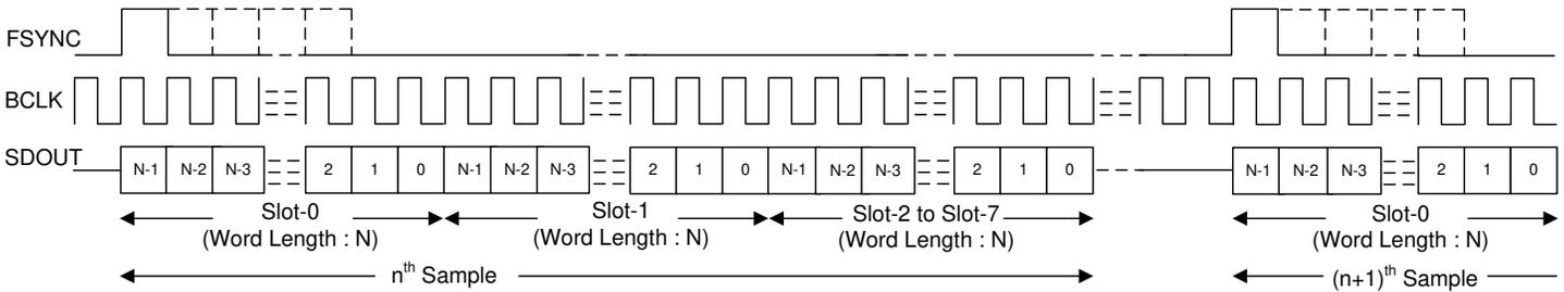
**Figure 6-1. TDM Mode Standard Protocol Timing (PASI\_TX\_OFFSET = 0)**
