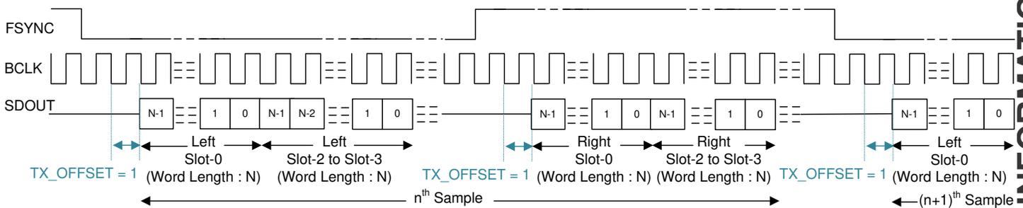
Figure 6-6. I<sup>2</sup>S Protocol Timing (PASI\_TX\_OFFSET = 1)
