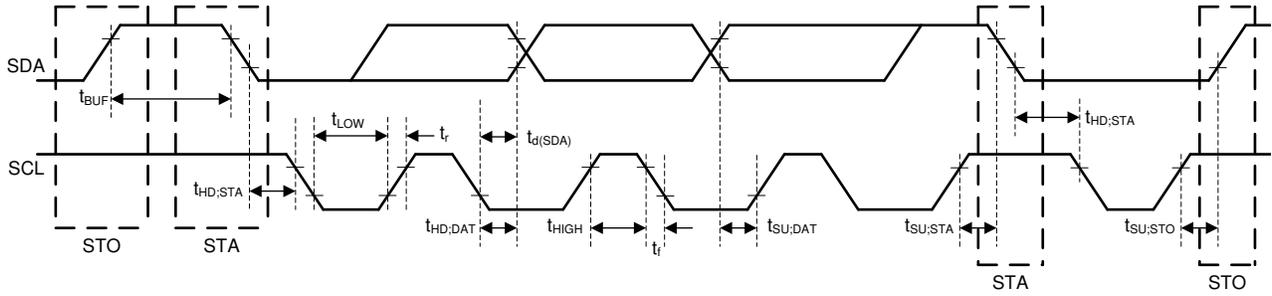
Figure 5-1. I<sup>2</sup>C Interface Timing Diagram
