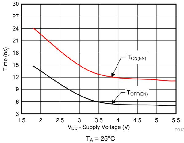
Figure 5-13.  $T_{ON(EN)}$  and  $T_{OFF(EN)}$  vs Supply Voltage
