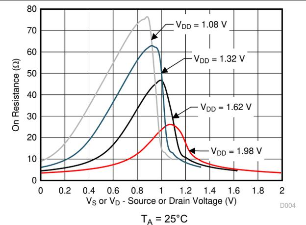
Figure 5-4. On-Resistance vs Source or Drain Voltage
