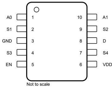
**Figure 4-1. DGS Package, 10-Pin VSSOP (Top View)**
