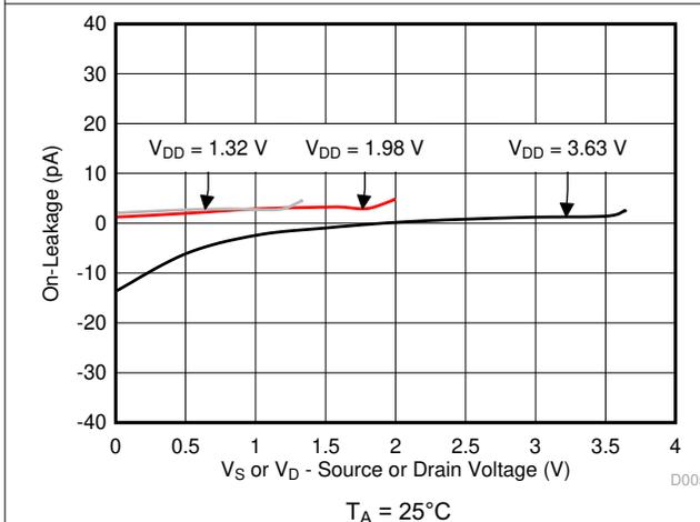
Figure 5-5. On-Leakage vs Source or Drain Voltage
