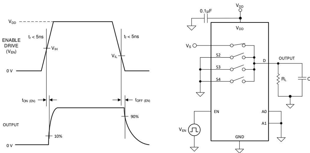
Figure 6-6. Turn-On and Turn-Off Time Measurement Setup
