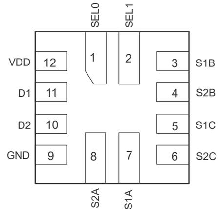
Figure 5-2. RMG Package, 12-Pin VQFN (Bottom View)
