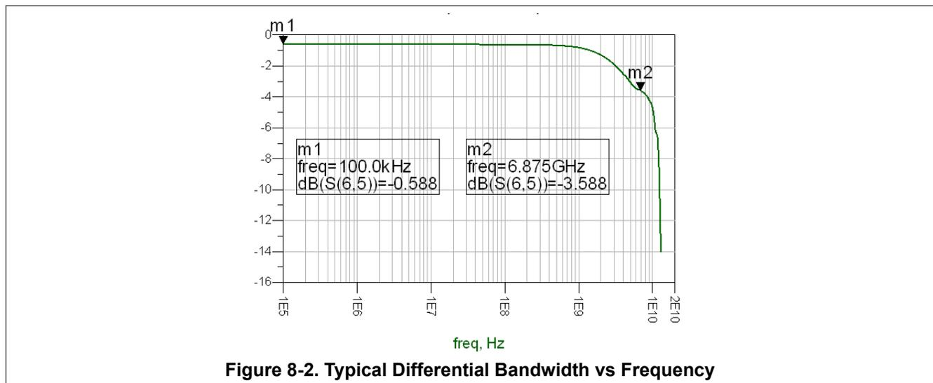
**Figure 8-2. Typical Differential Bandwidth vs Frequency**
