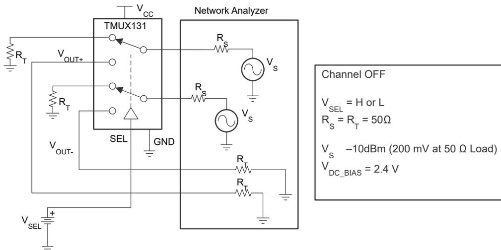
Figure 7-3. Differential Off-Isolation ( $O_{ISO}$ )
