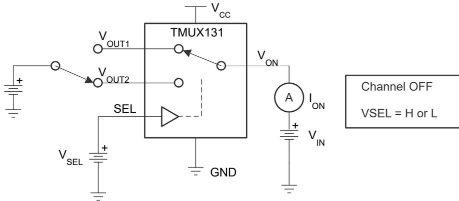
Figure 7-2. OFF Leakage Current ( $I_{OZ}$ )
