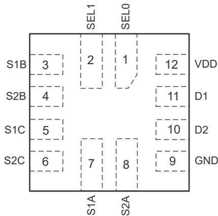
Figure 5-1. RMG Package, 12-Pin VQFN (Top View)
