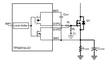
Figure 7-4. Inrush Current Limiting Using G1 Gate Drive
