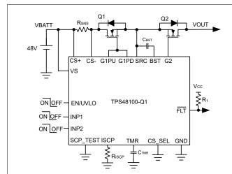
Figure 7-5. TPS48100-Q1 Application Circuit With External Sense Resistor RSNS Based High Side Current Sensing
