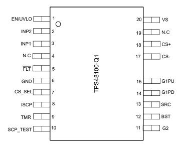
Figure 4-1. DGX Package, 19-Pin VSSOP (Top View)
