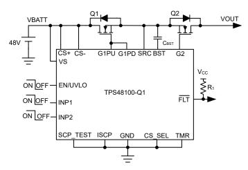
Figure 7-11. TPS48100-Q1 Application Circuit for Simple Gate Driver
