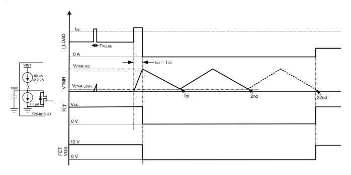
Figure 7-8. Short-Circuit Protection With Auto-Retry
