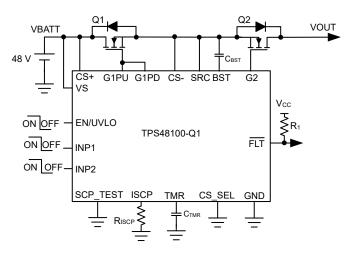
Figure 7-7. TPS48100-Q1 Application Circuit with MOSFET RDSON Based Current Sensing
