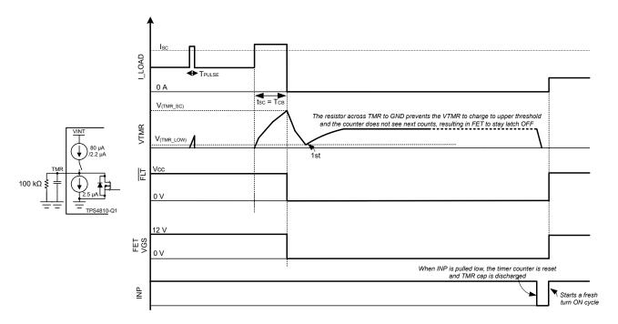
Figure 7-9. Short-Circuit Protection With Latch-Off
