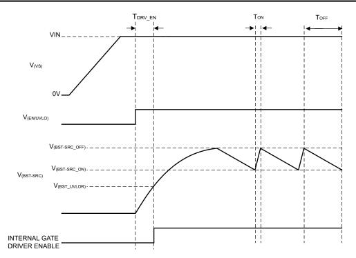
Figure 7-2. Charge Pump Operation
