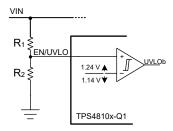
Figure 7-10. Programming Undervoltage Protection
