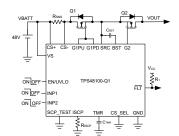
**BMS Breaker With Separate Discharge and Charge FET Control**
