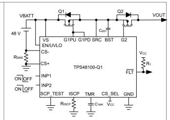
Figure 7-6. TPS48100-Q1 Application Circuit With External Sense Resistor RSNS Based Low Side Current Sensing
