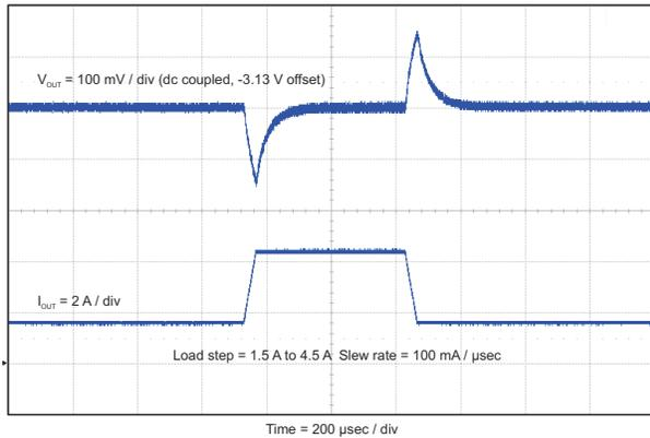
**Figure 8-2. Load Transient**
