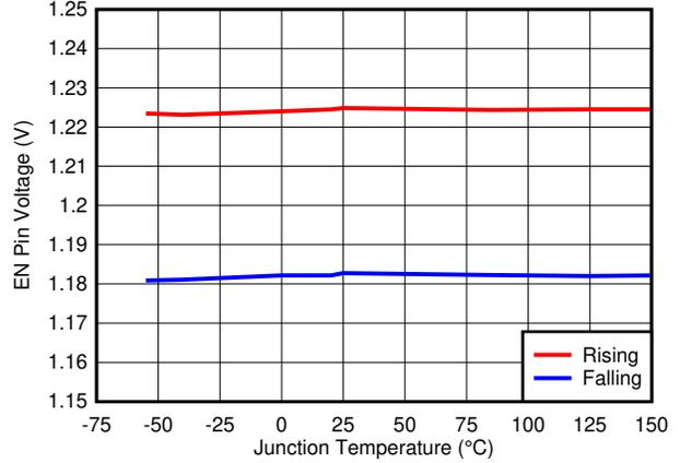
Figure 6-8. EN Pin UVLO Threshold vs Temperature
