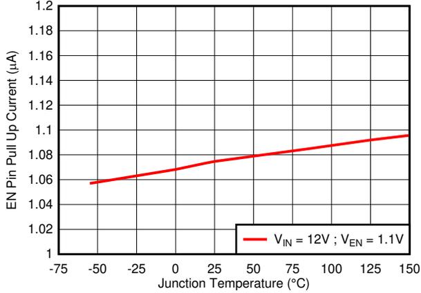
Figure 6-7. EN Pin Pullup Current vs Temperature
