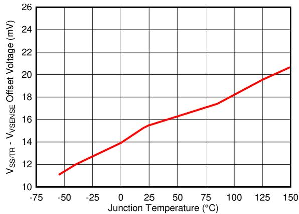
Figure 6-11. (SS/TR - VSENSE) Offset vs Temperature
