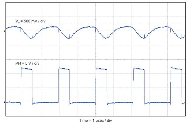
**Figure 8-7. Input Voltage Ripple With Full Load**
