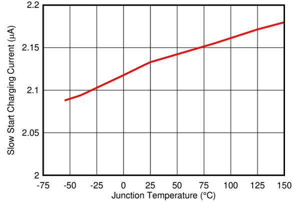
Figure 6-10. Slow Start Charge Current vs Temperature
