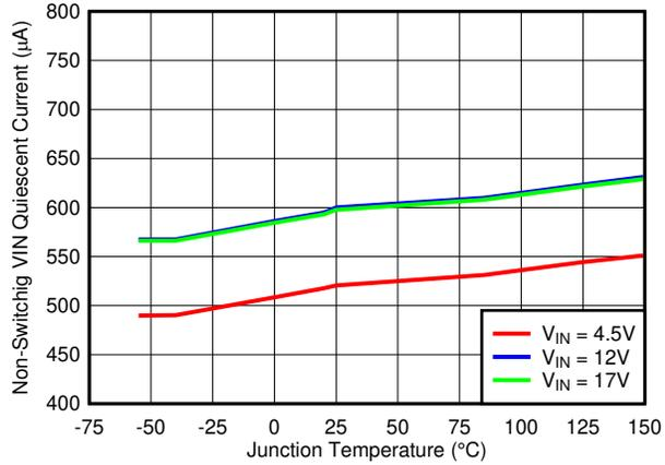
Figure 6-9. Non-Switching Operating Quiescent Current vs Temperature
