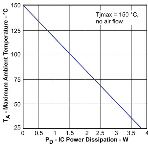
**Figure 8-16. Maximum Ambient Temperature vs IC Power Dissipation**
