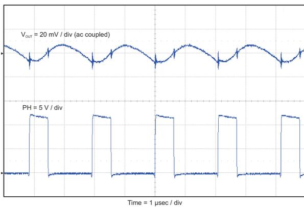
**Figure 8-6. Output Voltage Ripple With No Load**
