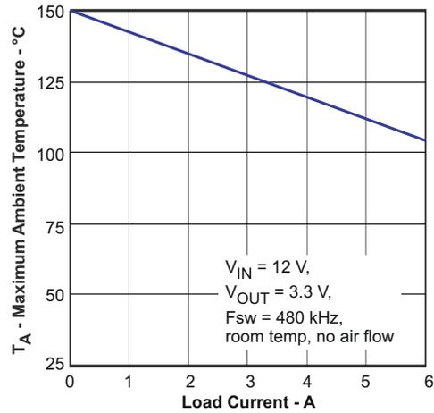
**Figure 8-15. Maximum Ambient Temperature vs Load Current**
