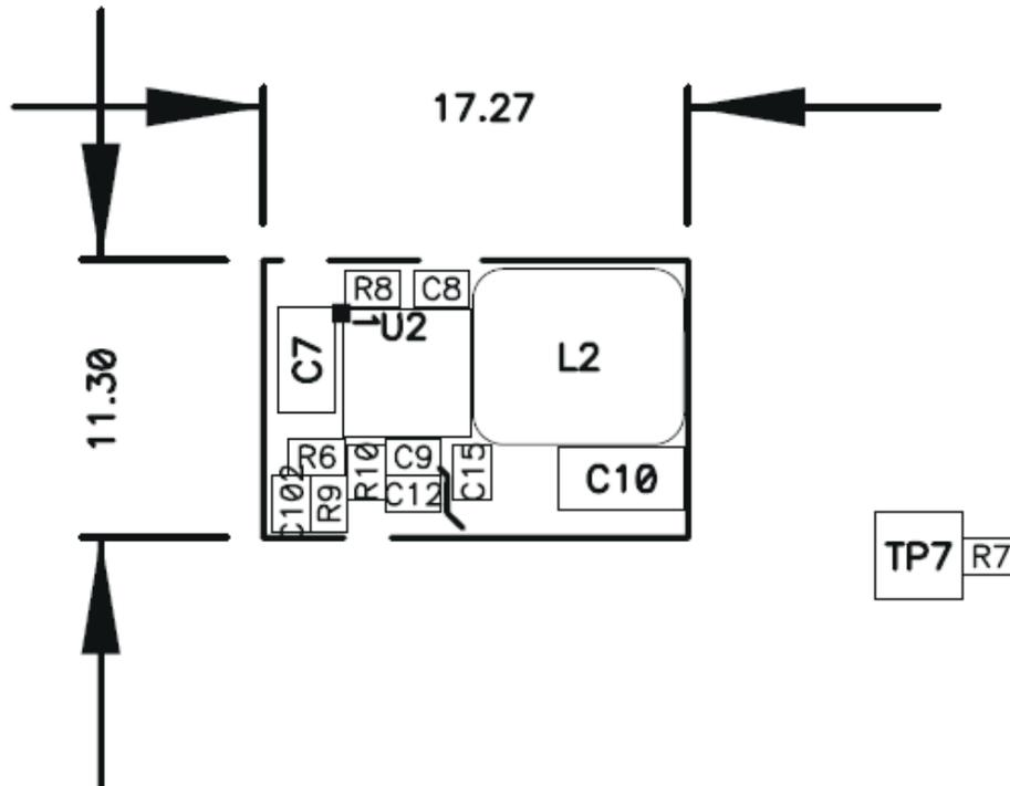
Figure 10-2. Ultra-Small PCB Layout Using TPS54622-EP (PMP4854-2)
