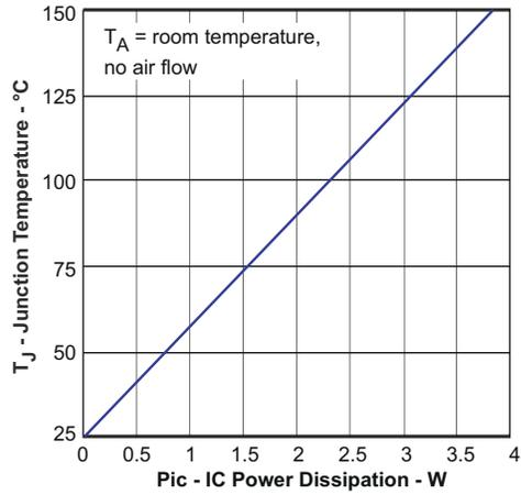
**Figure 8-14. Junction Temperature vs IC Power Dissipation**
