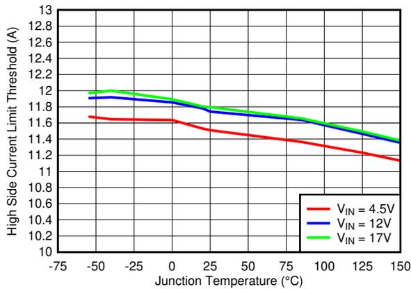
Figure 6-13. High-Side Current Limit Threshold vs Temperature
