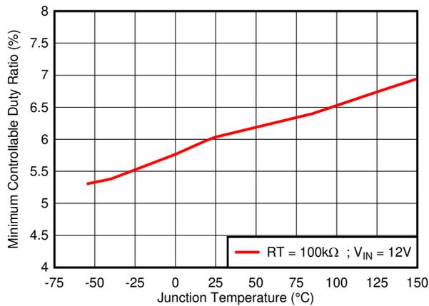
Figure 6-15. Minimum Controllable Duty Ratio vs Temperature
