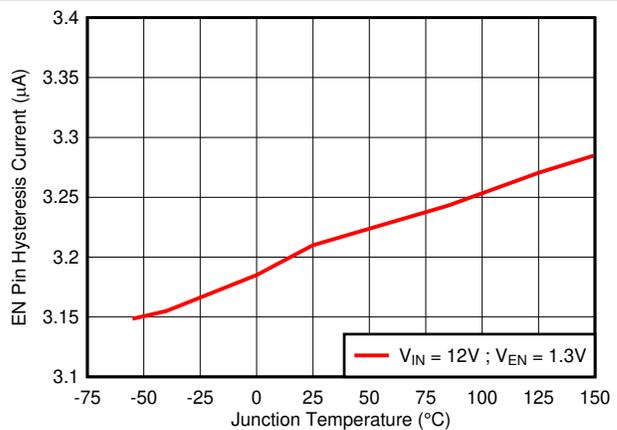
Figure 6-6. EN Pin Hysteresis Current vs Temperature
