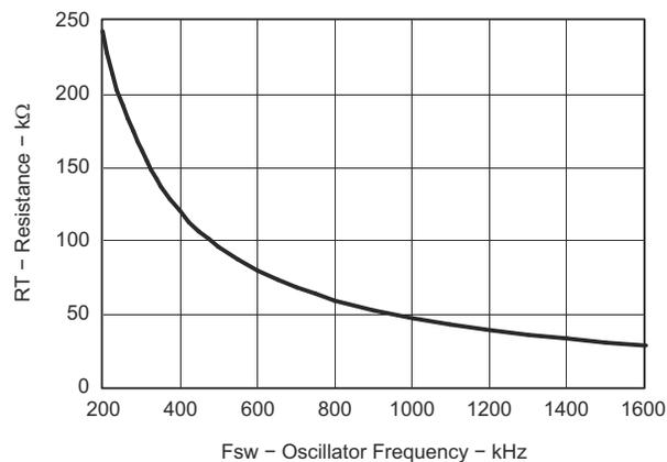
**Figure 7-8. RT Set Resistor vs Switching Frequency**
