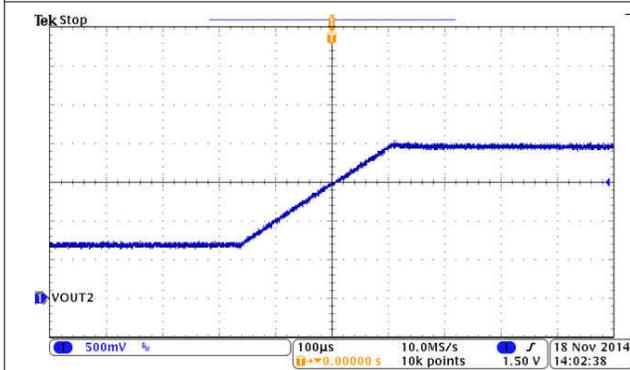
**Figure 8-19. VID2 from 00 to 7F, SR = 10 mV/Cycle**
