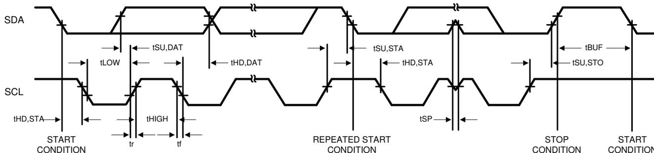
**Figure 7-14. I<sup>2</sup>C Interface Timing Diagram**
