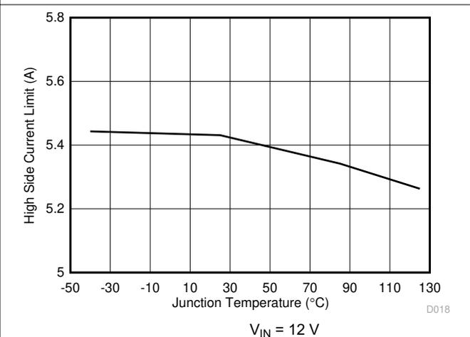
Figure 6-18. Buck1 High-Side Current Limit vs Temperature
