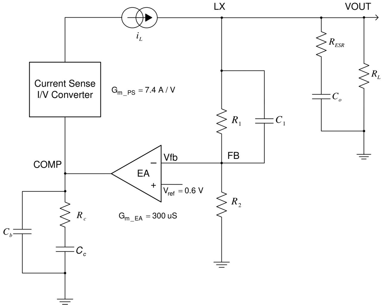
**Figure 8-2. DC/DC Loop Compensation**
