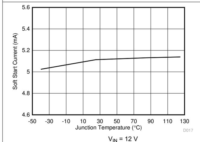
Figure 6-17. SS Pin Charge Current vs Temperature
