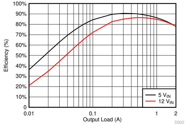
Figure 6-2. BUCK2 Efficiency
