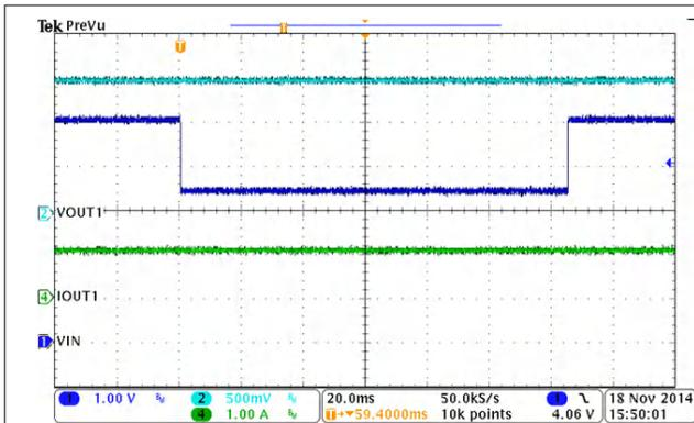
**Figure 8-23. Operation at VIN Drop to 2.5 V**
