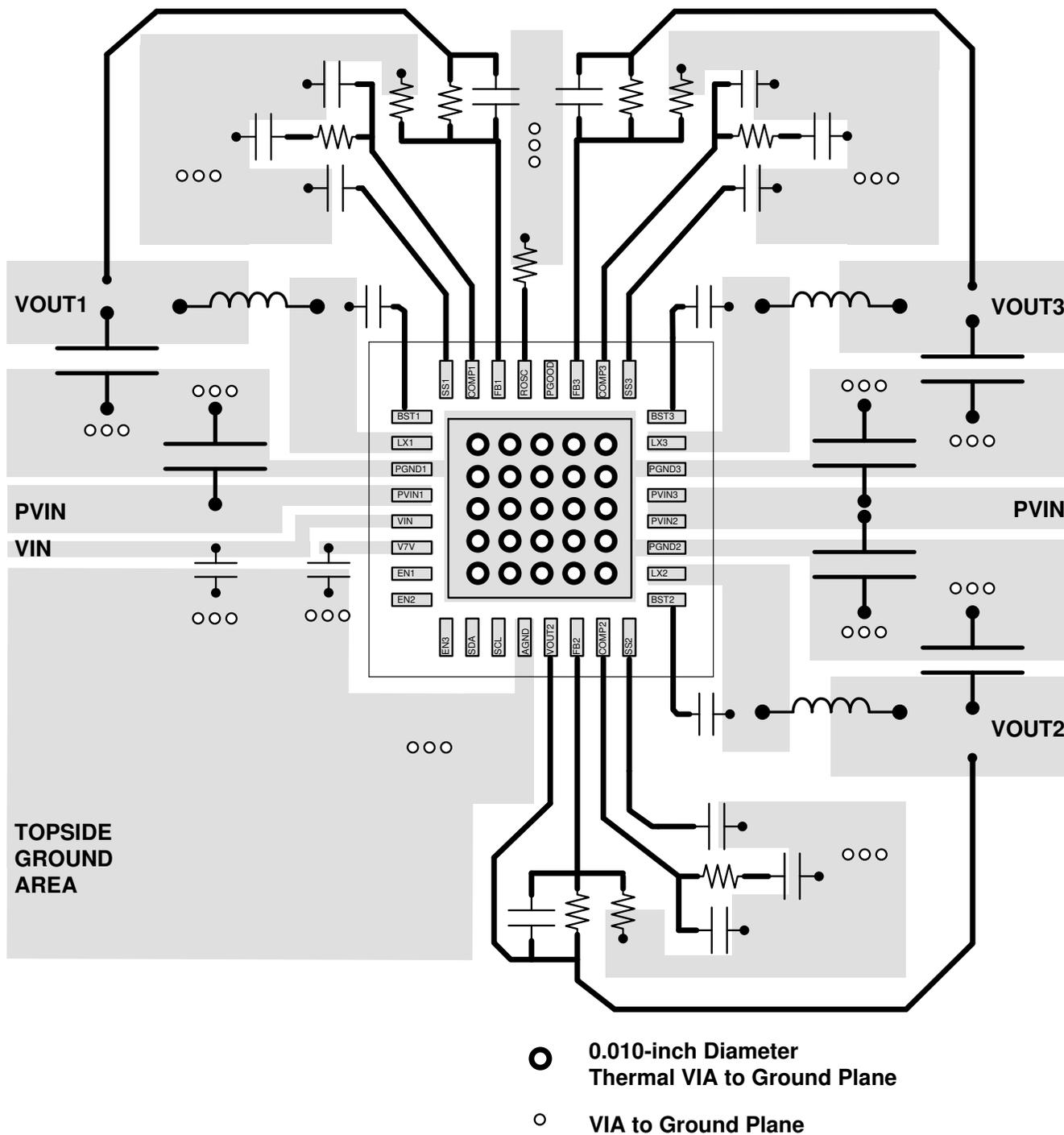
Figure 8-25. PCB Layout
