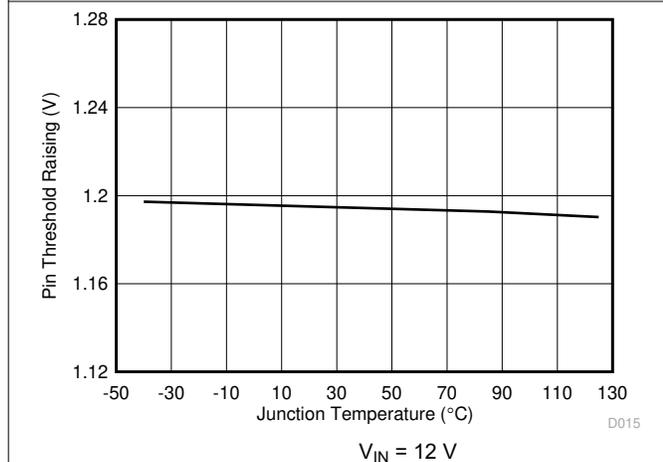
Figure 6-15. EN Pin Threshold Rising vs Temperature
