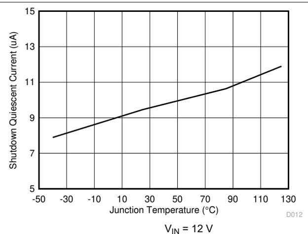
Figure 6-12. Shutdown Quiescent Current vs Temperature
