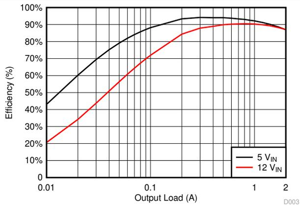
Figure 6-3. BUCK3 Efficiency
