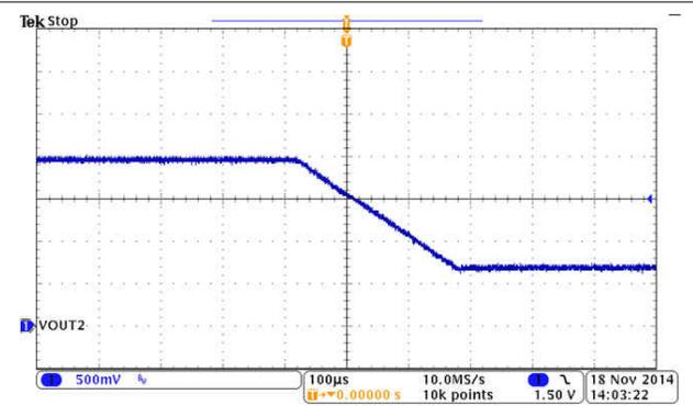
**Figure 8-20. VID2 from 7F to 00, SR = 10 mV/Cycle**
