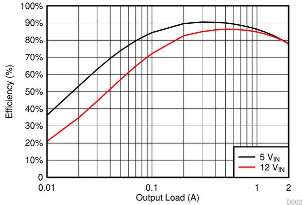
Figure 6-1. BUCK1 Efficiency
