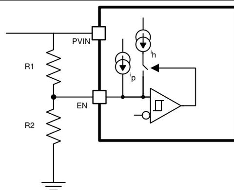
**Figure 7-4. Adjustable PVIN UVLO, VIN > 4 V**
