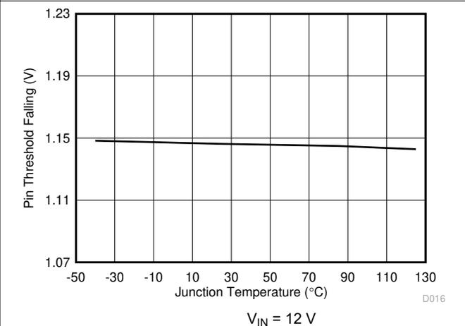
Figure 6-16. EN Pin Threshold Falling vs Temperature
