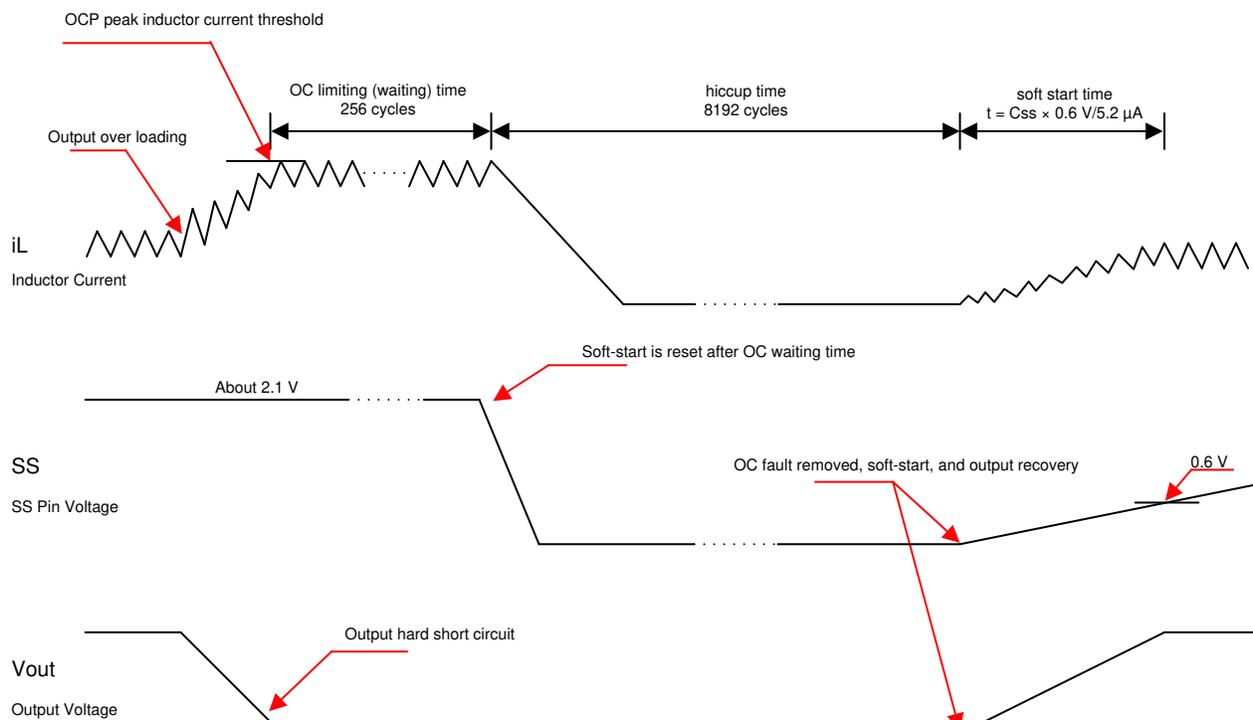
**Figure 7-11. Overcurrent Protection**
