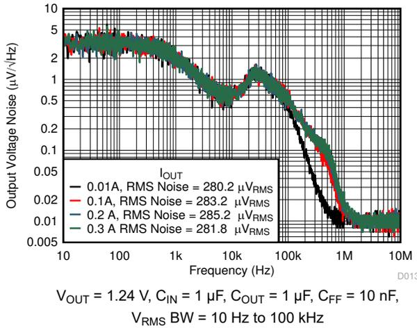
Figure 7-25. Output Noise ( $V_n$ ) vs Frequency and  $I_{OUT}$
