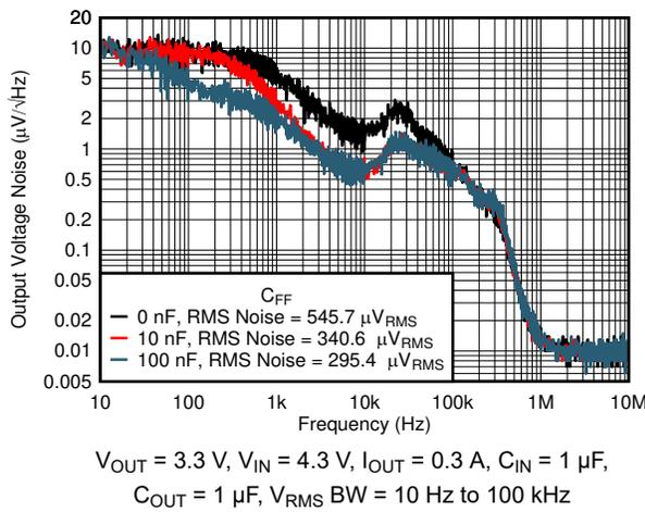
Figure 7-27. Output Noise ( $V_n$ ) vs Frequency and  $C_{FF}$
