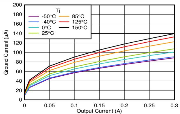
Figure 7-12.  $I_{GND}$  vs  $I_{OUT}$
