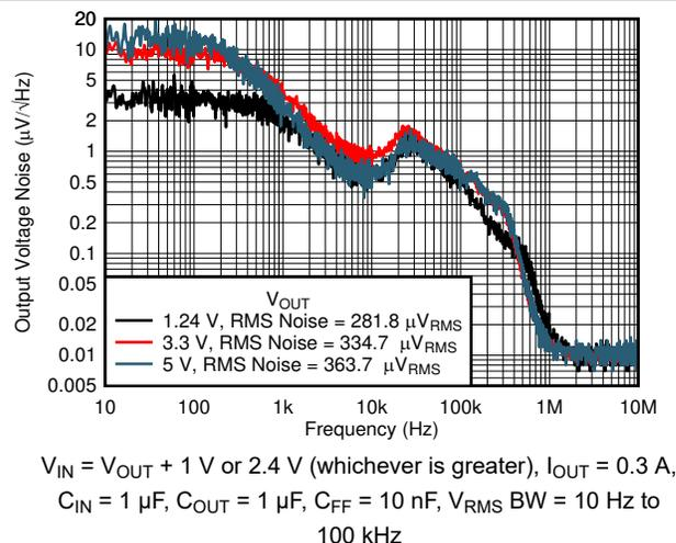
Figure 7-24. Output Noise ( $V_n$ ) vs Frequency and  $V_{OUT}$
