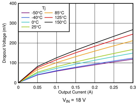
Figure 7-7. Dropout Voltage vs  $I_{OUT}$
