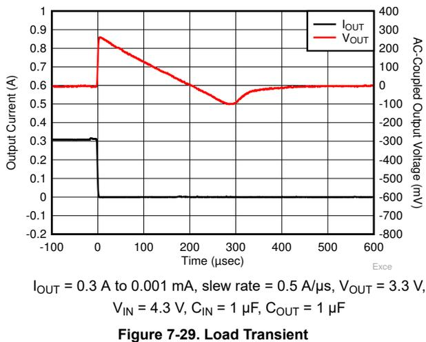
Figure 7-29. Load Transient
