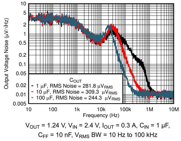
Figure 7-26. Output Noise ( $V_n$ ) vs Frequency and  $C_{OUT}$
