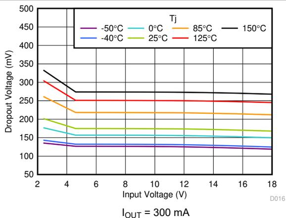
Figure 7-5. Dropout Voltage vs  $V_{IN}$
