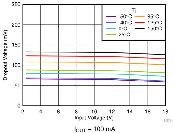
Figure 7-3. Dropout Voltage vs  $V_{IN}$
