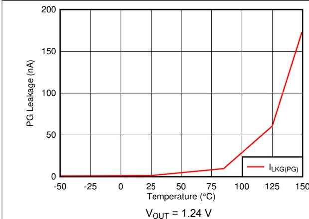
Figure 7-17. PG Leakage Current vs Temperature
