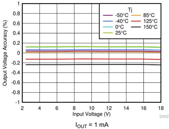
Figure 7-1. Line Regulation vs  $V_{IN}$
