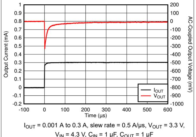
Figure 7-28. Load Transient
