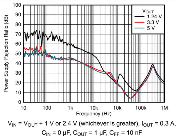
Figure 7-23. PSRR vs Frequency and  $V_{OUT}$
