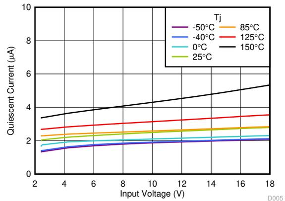
Figure 7-10.  $I_Q$  vs  $V_{IN}$
