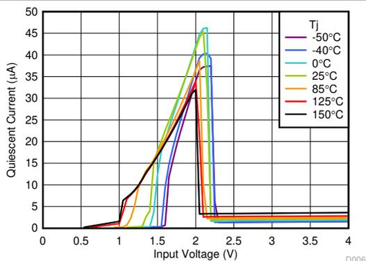
Figure 7-11.  $I_Q$  vs  $V_{IN}$
