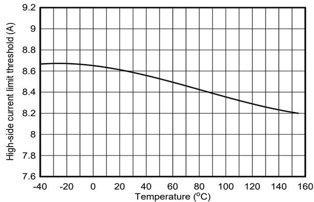
Figure 5-3. High-Side Current Limit Threshold vs Temperature
