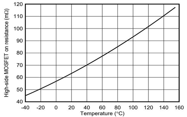
Figure 5-2. High-Side MOSFET On Resistance vs Temperature
