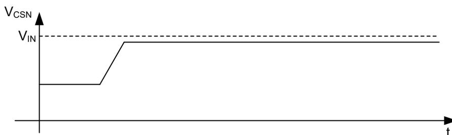
**Figure 6-10. Open-Circuit Condition with Minimum Off-Time Operation**
