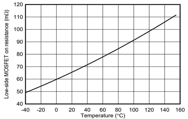
Figure 5-4. Low-Side MOSFET On Resistance vs Temperature
