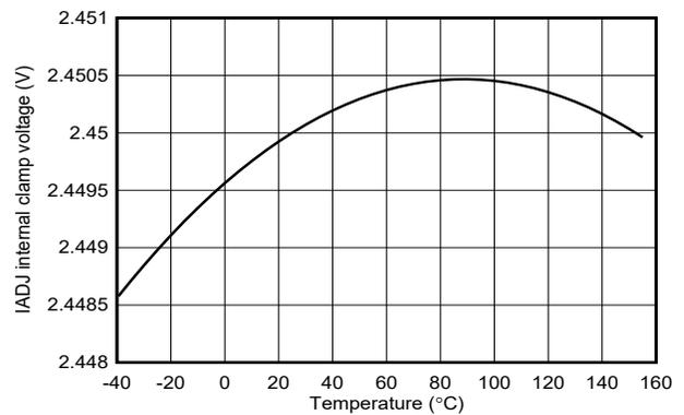
Figure 5-6. IADJ Internal Clamp Voltage vs Temperature
