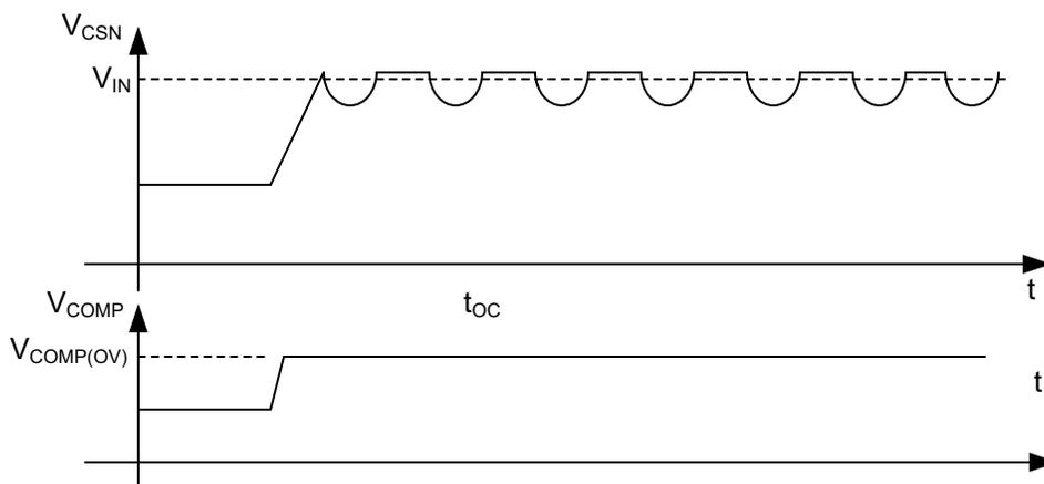
**Figure 6-9. Open-Circuit Condition with Output Voltage Oscillation**
