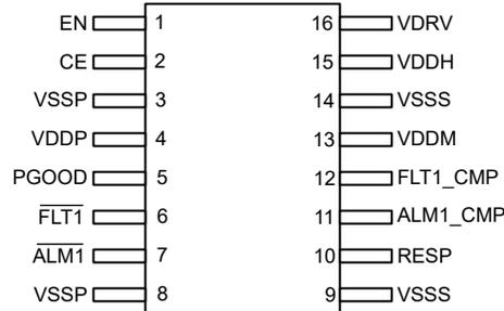
**Figure 5-4. TPSI313x-Q1 DVX Package, 16-Pin SSOP (Top View)**
