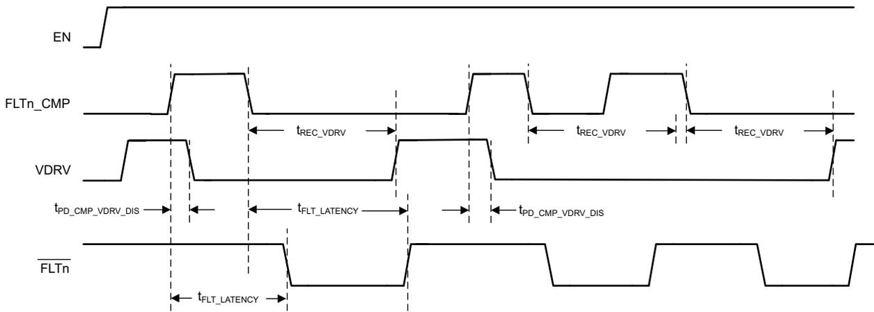
Figure 7-2. VDRV Auto-Recovery Timing (CE = 1 or CE = VDDP)
