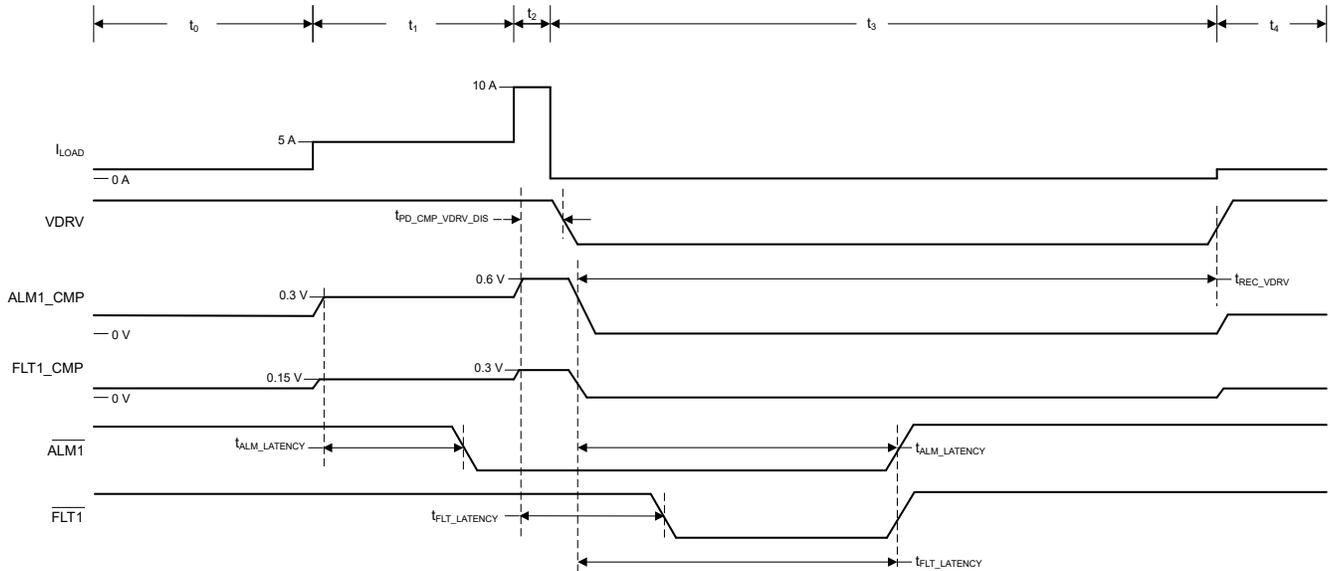
Figure 9-2. Over-current protection typical timing and behavior
