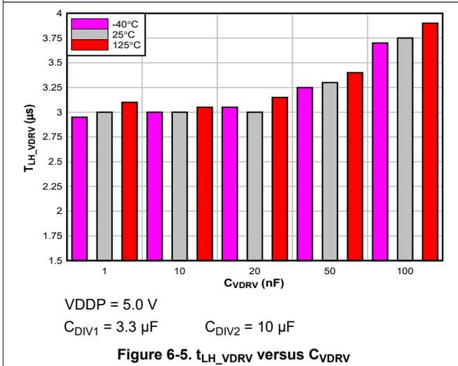
Figure 6-5. t<sub>LH\_VDRV</sub> versus C<sub>VDRV</sub>
