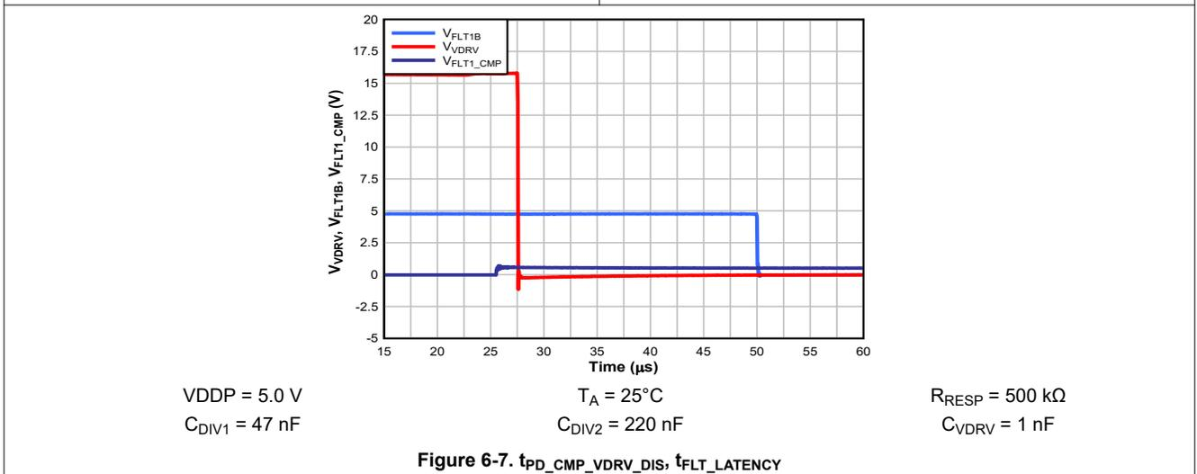
Figure 6-7. t<sub>PD\_CMP\_VDRV\_DIS</sub>, t<sub>FLT\_LATENCY</sub>
