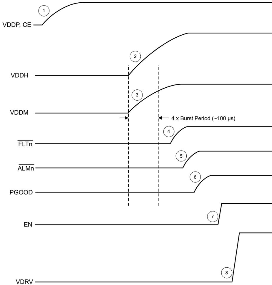
Figure 8-10. TPSI310x-Q1 Typical Start-up (CE = VDDP,  $\overline{\text{FLTn\_CMP}} = 0$ ,  $\overline{\text{ALMn\_CMP}} = 0$ )
