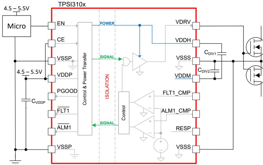
Figure 8-9. Simplified Schematic
