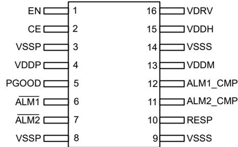
Figure 5-3. TPSI312x-Q1 DVX Package, 16-Pin SSOP (Top View)
