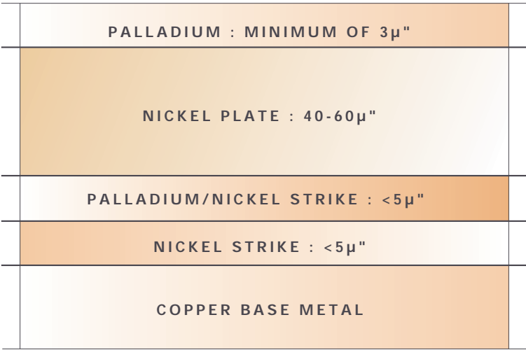
FIGURE 1 : Structure of TI Palladium Lead Finish
