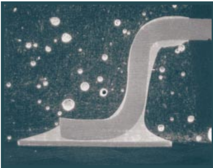
FIGURE 35 : Solder Wicking on Solder Plated Lead
