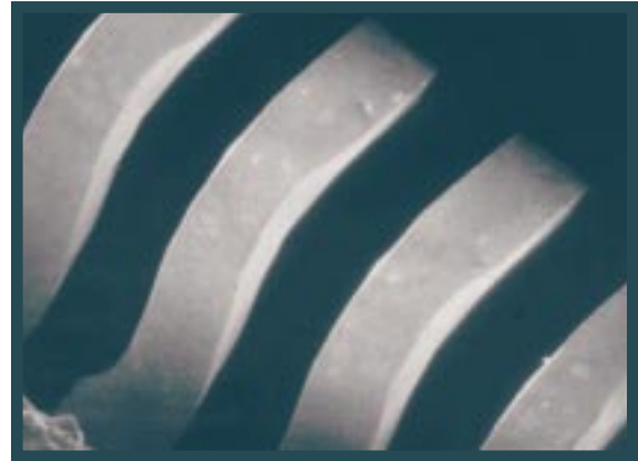
FIGURE 14 : Good Solderability Results With no Bridging on 120 pin TQFP Package Tested With SMT Method
