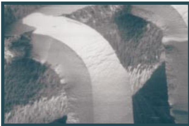
FIGURE 20 : Surface Cracks on SOIC Shoulder {77X}
