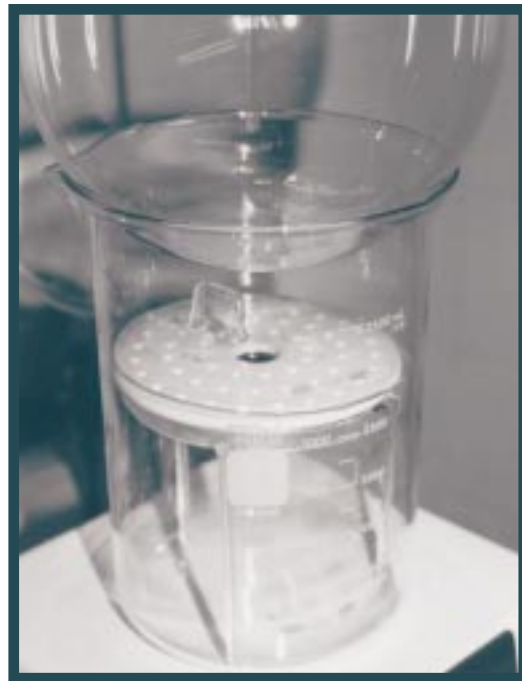
FIGURE 4 : Close up of Beaker Steam Age Set-up
