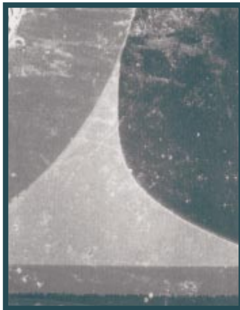
FIGURE 30 : Palladium Plated SOIC Device, No-clean Solder Paste E4
