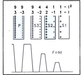
Fig. 14 - Passive Winding Losses
