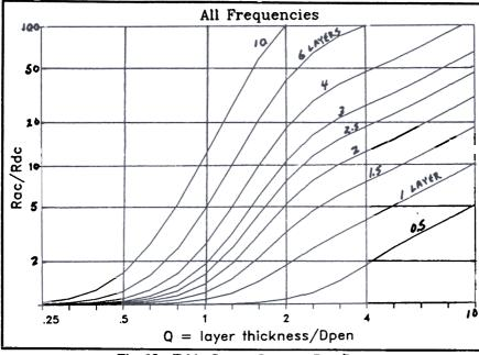
substituted for the original wire (taking care to handle this properly), there will be 40 wires, 20 per layer, 2 layers deep. Q is now 2. Entering Fig. 15 at Q=2 and 2 layers, F<sub>R</sub> is 5.2 -- it went up! The reason for this is the wire size is still too large for effective penetration and cancellation of the eddy currents, and the number of lavers has been doubled with the extra eddy current surfaces this generates.
