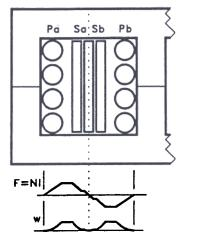
Fig. 11 - Interleaved Windings
