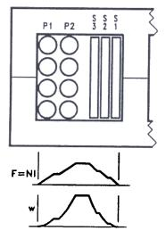
Fig. 10 - Multiple Layer Winding
