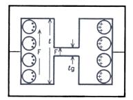
Fig. 8 - Inductor Winding
