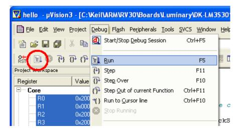
4. The application starts running, and you should see the text "Hello World!" output to the OLED display of the evaluation board.
