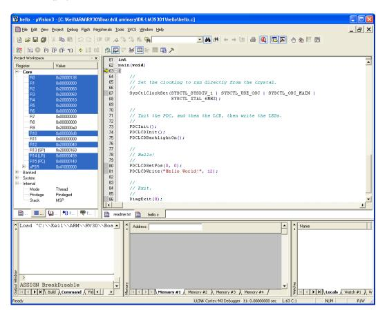
3. From here, you can examine and modify memory, program variables and processor registers, set breakpoints, single step, and all other typical debugging activities. To run the program, select "Run" from the Debug menu, or click on the "Run" button (icon).
