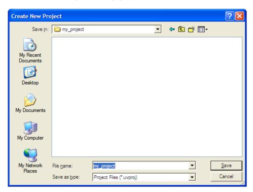
Once the project file (.uvproj) is saved, a dialog window pops up asking you to select the device that you are using. Select the appropriate device under the Luminary Micro or Texas Instruments list.
