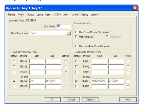
Here you need to set up the Xtal frequency for your specific board. This step is important because the value of the Xtal field is used to calculate flash programming timing later on. Also check the ROM/RAM sizes to make sure that it corresponds to the device you have.
