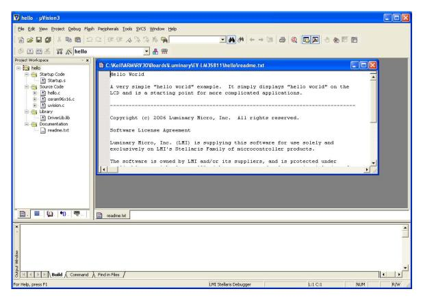
5. You can view source files in the project by double-clicking on a filename in the Project Workspace pane on the left. For example, double-click on hello.c, and the source file opens in the editor.
