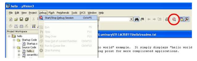
2. The IDE switches to debugging mode. The processor registers show up in a window on the left, the debugger command window is visible at the bottom, and the main window shows the source code being debugged. The debugger automatically stops at main.
