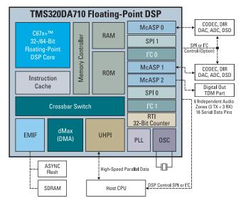
TMS320DA710 floating-point DSP block diagram
