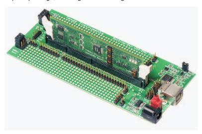
Figure 2. Retaining Clips
