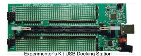
Figure 1. C2000 DIMM100 Experimenter's Kit
