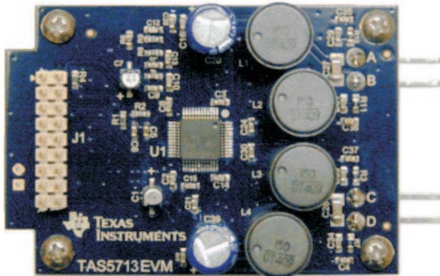
Figure 1. TAS5713EVM Printed-Circuit Board
