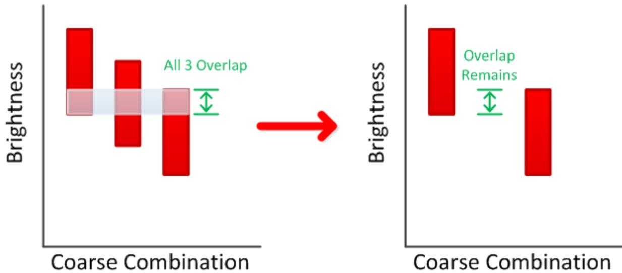
Figure 5-3. Removing heavily overlapping coarse combinations to decrease calibration time
