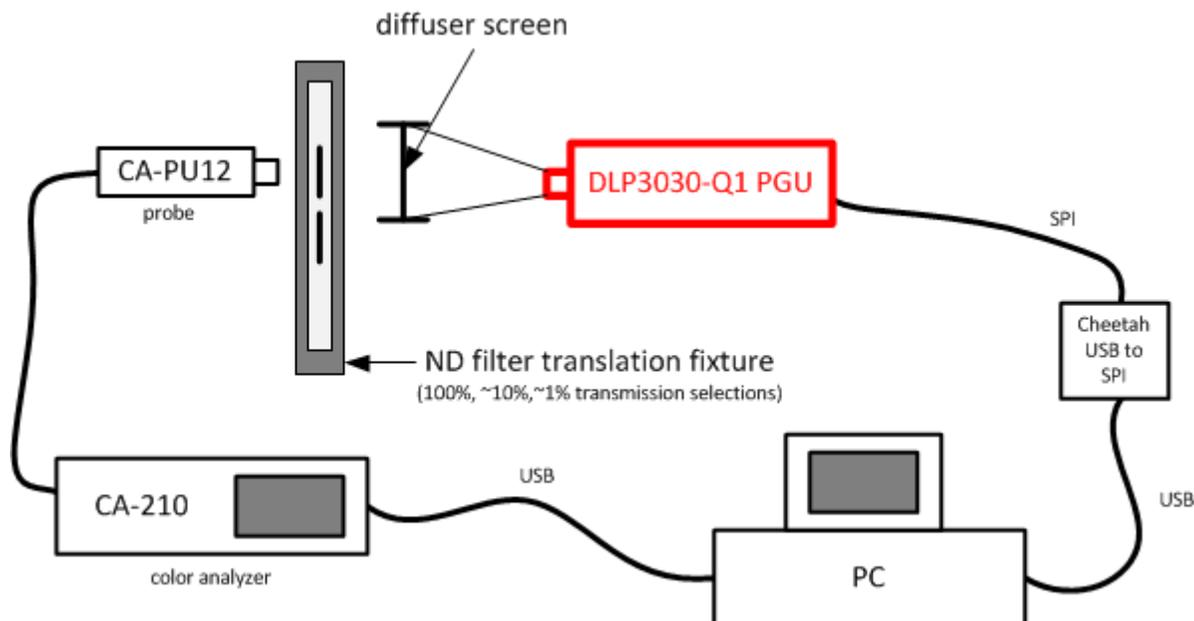
**Figure 3-1. Calibration Setup**
