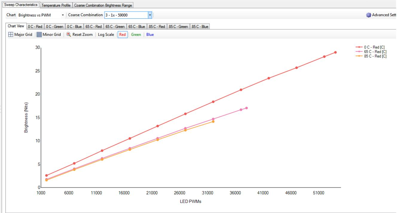
**Figure 6-7. Brightness Output vs LED PWM Value**
