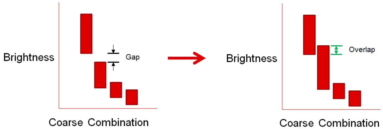
Figure 5-2. Closing brightness gaps between coarse combinations
