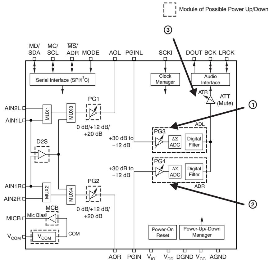
**Figure 3-6. EVM Modules Corresponding to Record Function**
