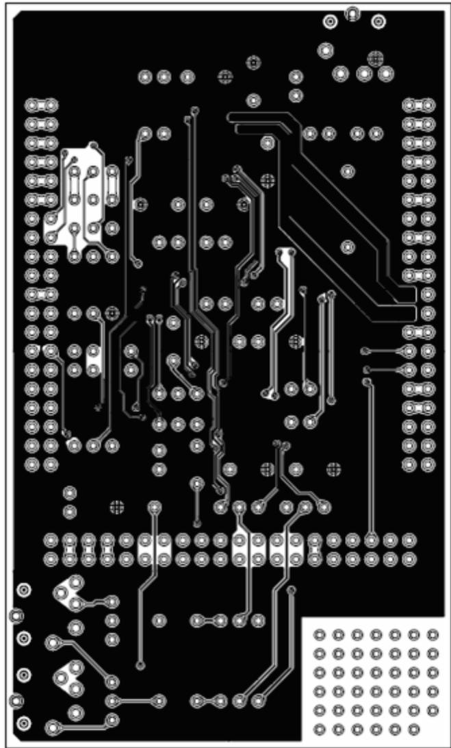
Figure 6-7. DEM-PCM1870RHF/1774RGP-A Board Layout—Solder Side
