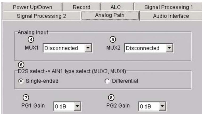
Figure 3-14. Analog Path Function Menu Tab
