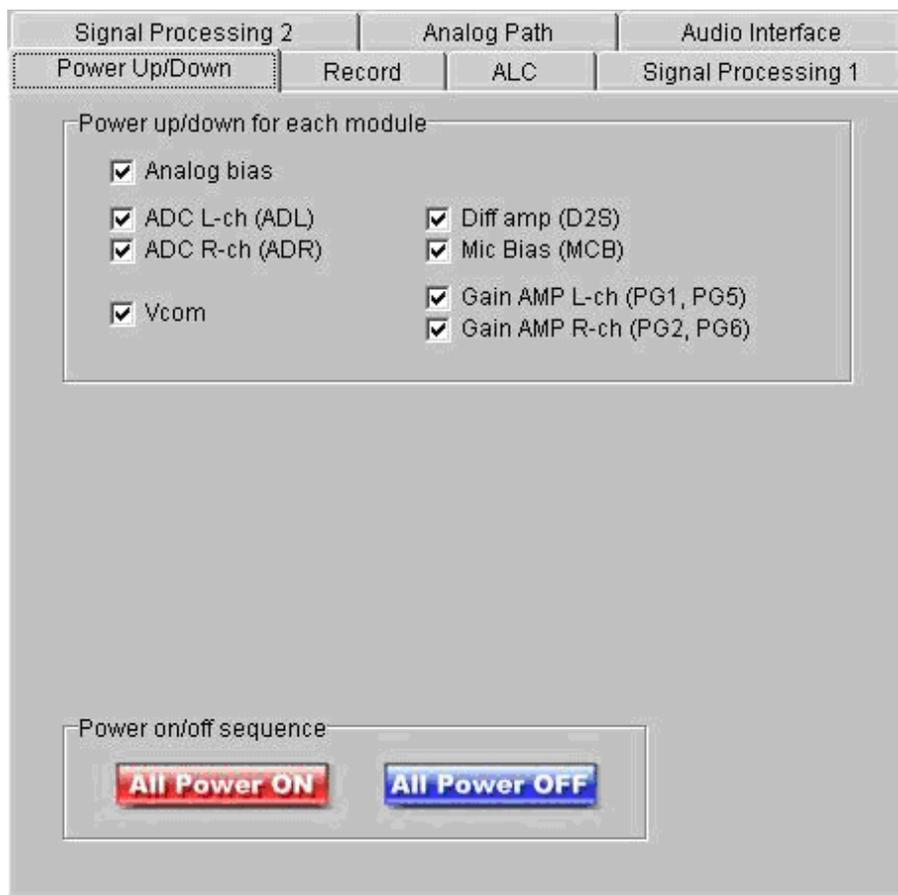
**Figure 3-4. Internal Module Power Up/Down Function Menu Tab**
