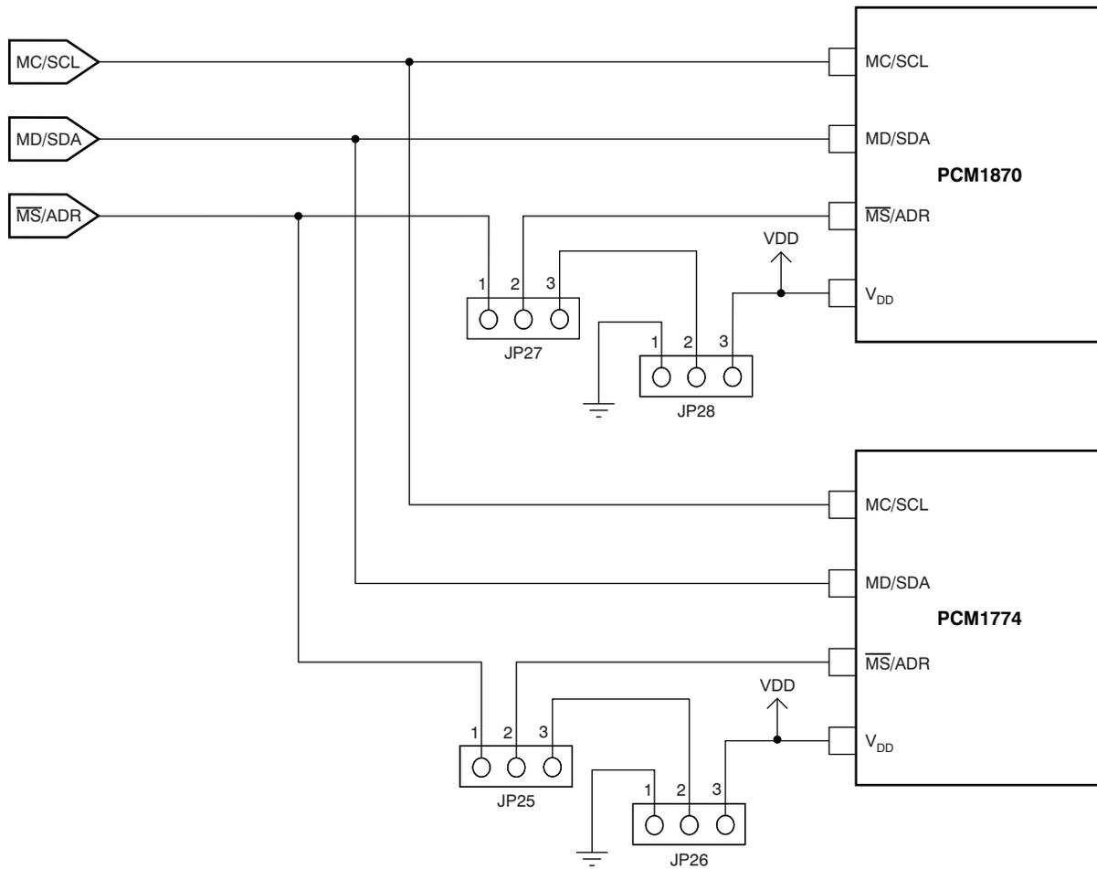
Figure 4-3.  $\overline{\text{MS}}/\text{ADR}$  Control Configuration for I<sup>2</sup>C Communication (Daughter Card #1)
