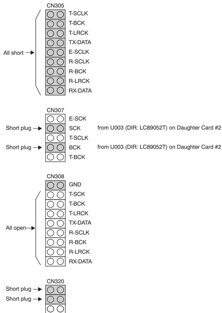
**Figure 5-2. Jumper Configuration for Slave Mode (Default)**
