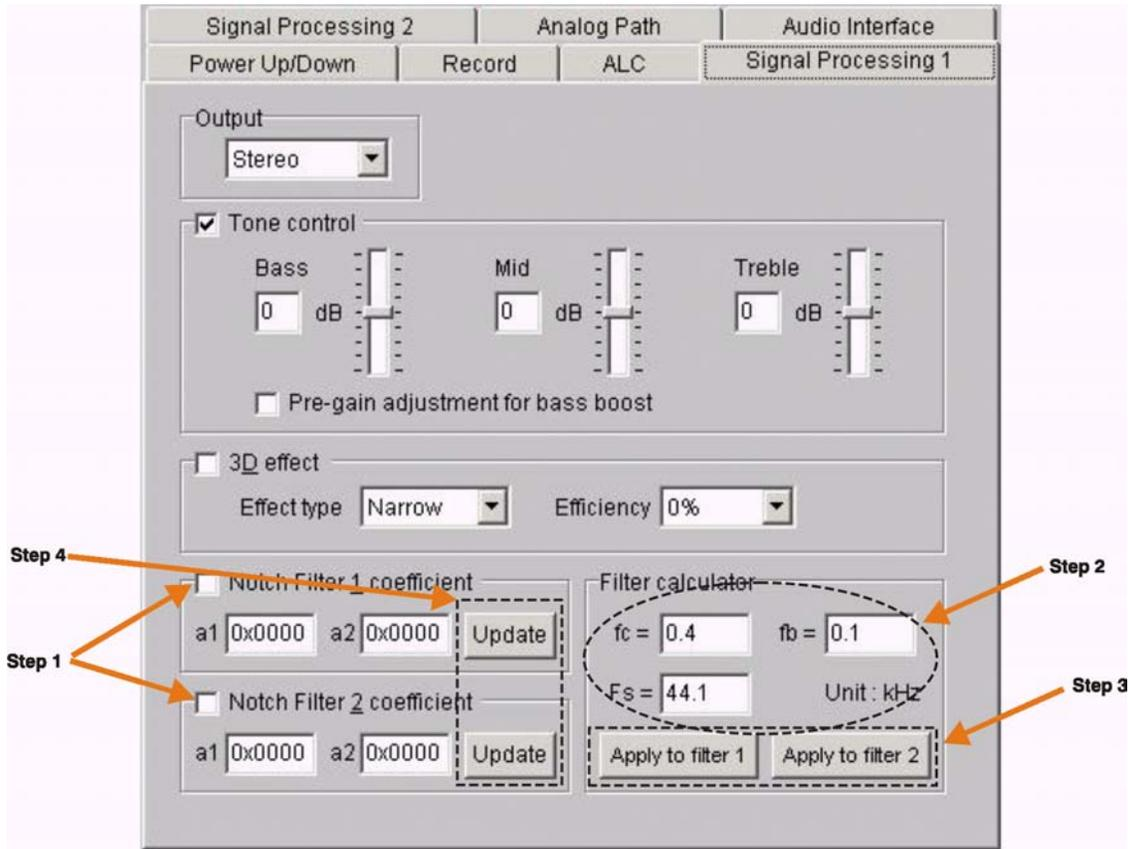
**Figure 3-9. Signal Processing 1 Function Menu Tab**
