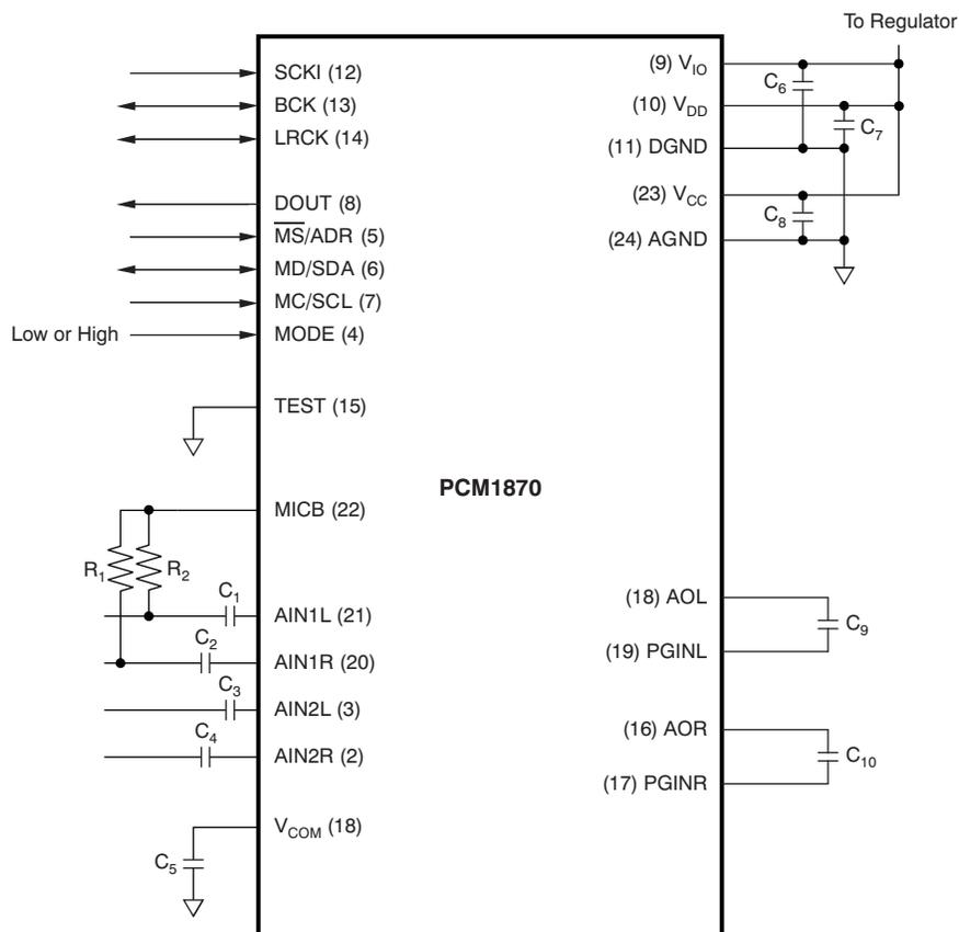
Figure 5-10. Basic Connection Diagram
