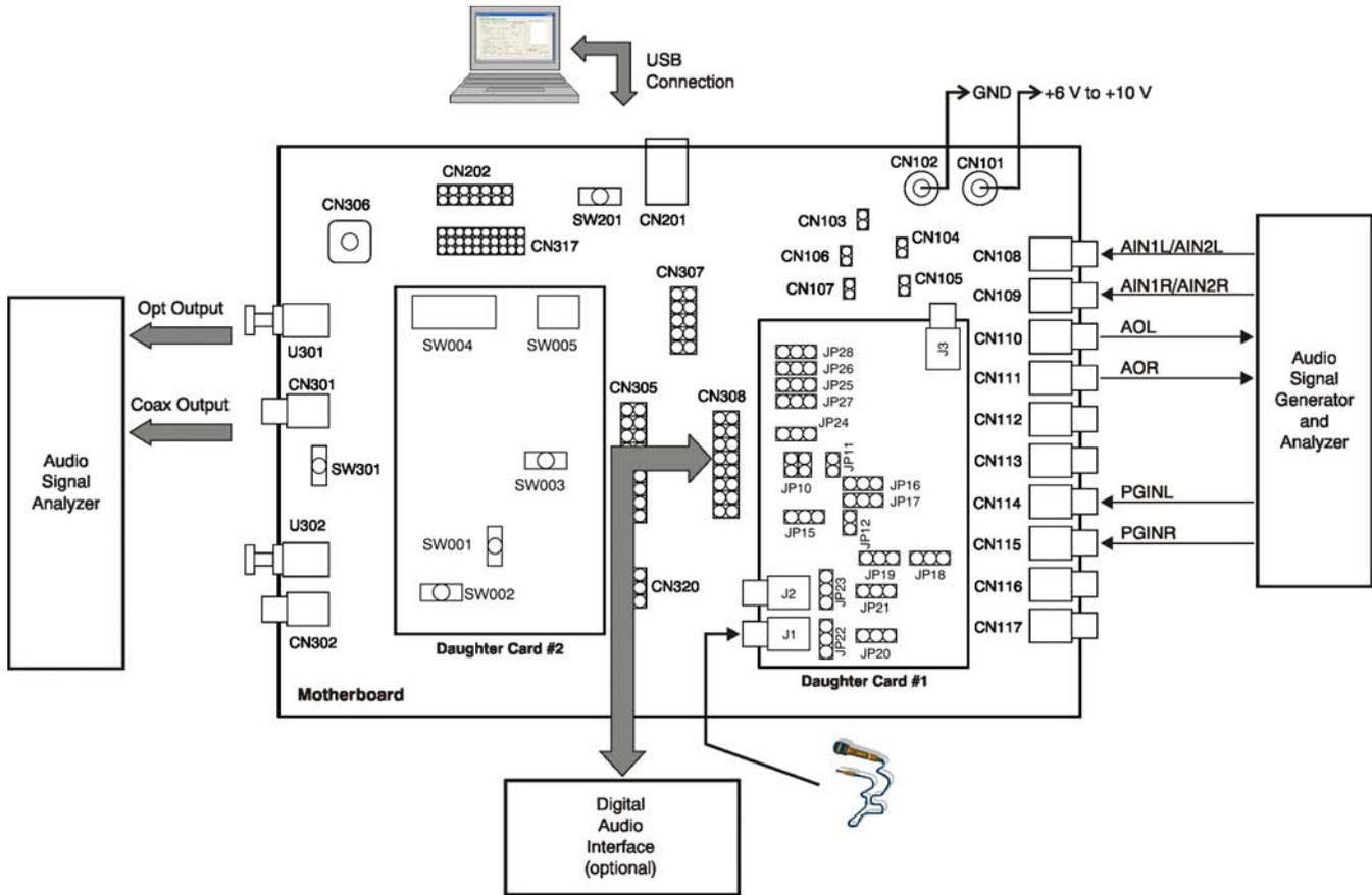
**Figure 2-2. EVM and External Equipment Connections**
