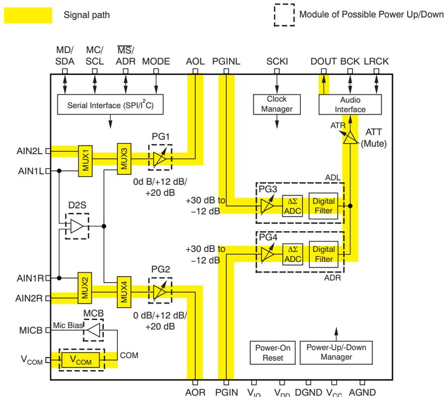
**Figure A-1. Line Input (AIN2L/AIN2R)**
