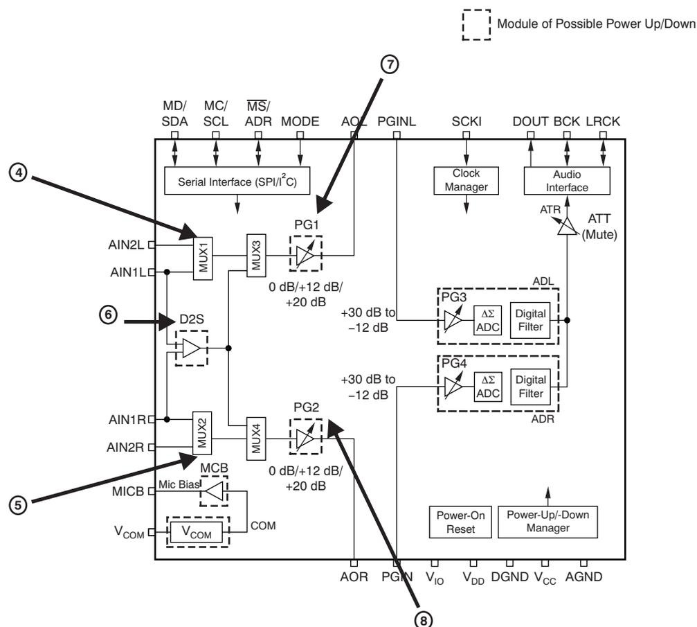
Figure 3-15. Modules Corresponding to Analog Path Function
