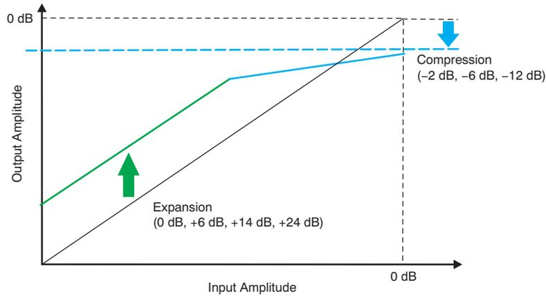
**Figure 3-8. ALC Compression and Expansion Characteristics**
