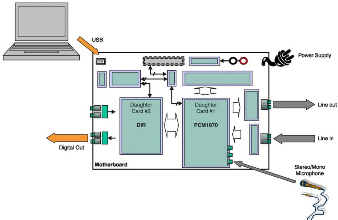
Figure 1-2. DEM-DAI1870 EVM System Diagram
