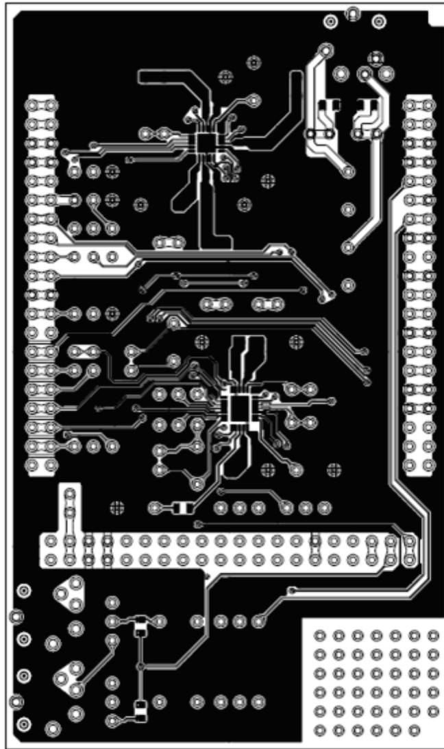
Figure 6-4. DEM-PCM1870RHF/1774RGP-A Board Layout—Component Side
