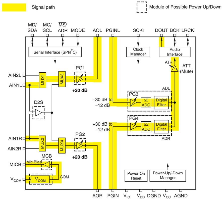
**Figure A-2. Microphone Input (AIN1L/AIN1R, +20 dB)**
