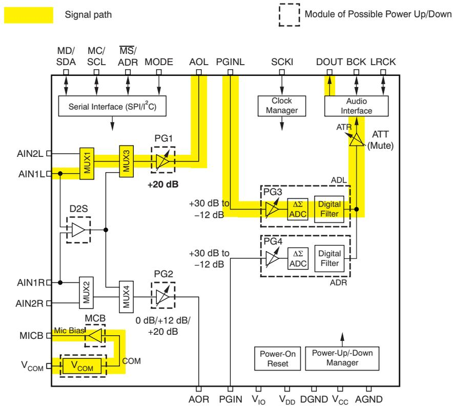
**Figure A-4. Mono Microphone Input (AIN1L, +20 dB)**
