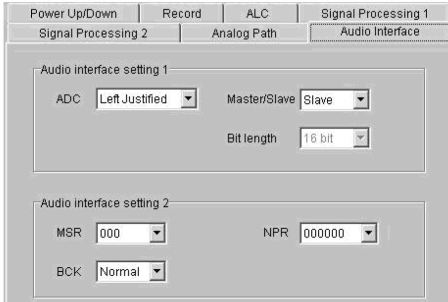
**Figure 3-16. Audio Interface Function Menu Tab**
