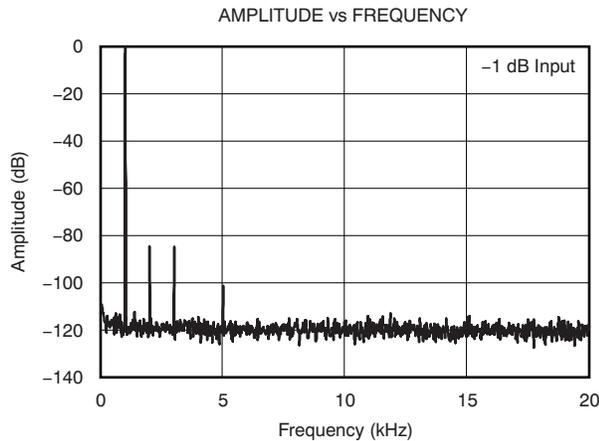
**Figure 5-7. ADC Amplitude vs Frequency
