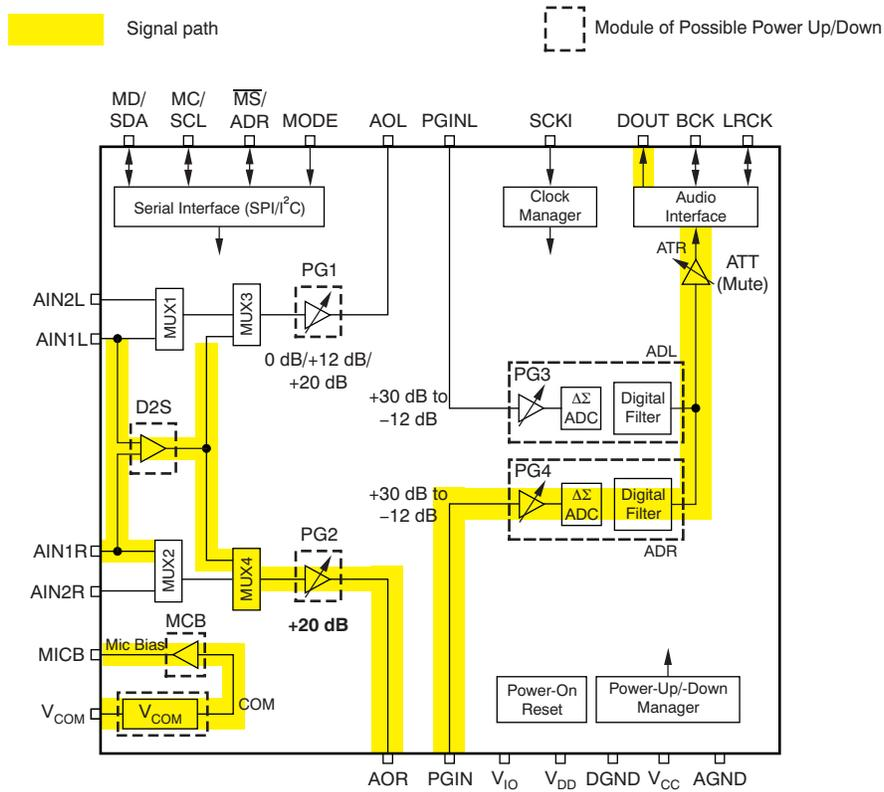
**Figure A-6. Mono Differential Microphone Input (AIN1L/AIN1R, +20 dB)**
