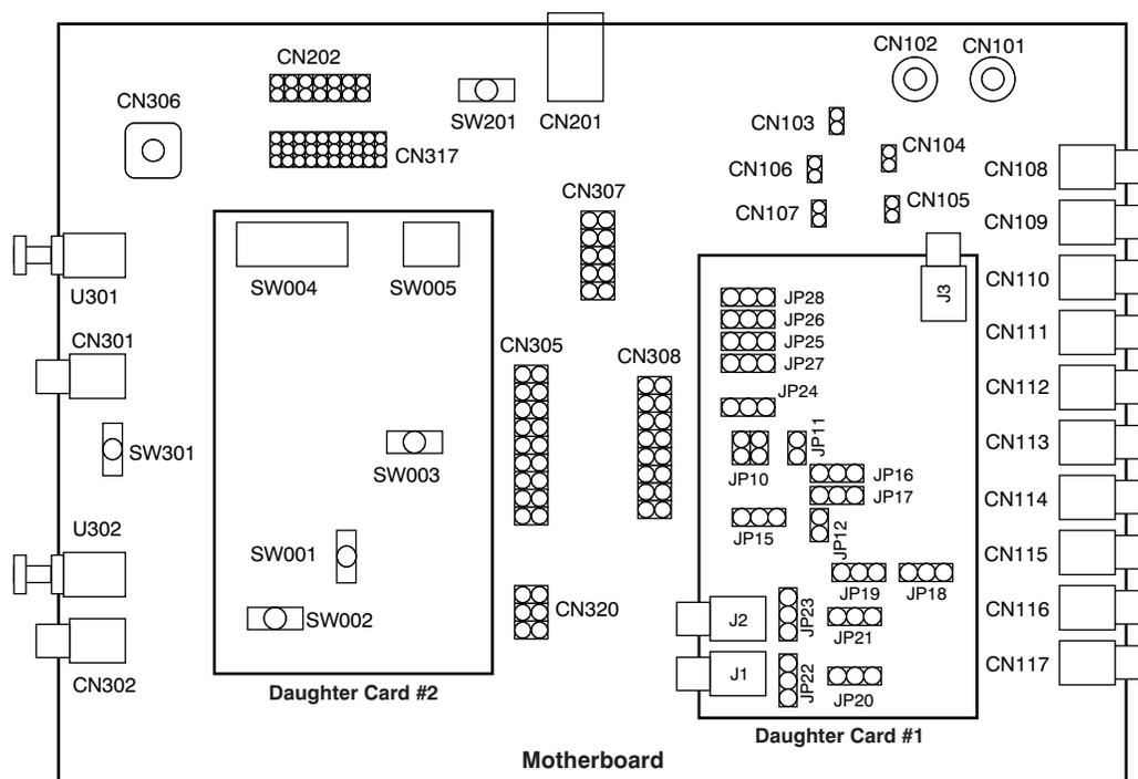
Note: Silkscreen symbol **CN320** is not printed on the motherboard, but it is located in the position described.
