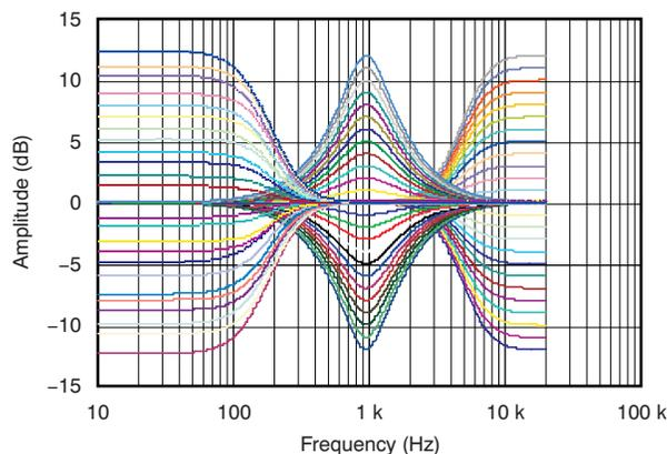
**Figure 3-10. Three-Band Tone Control (Bass, Mid, Treble)**
