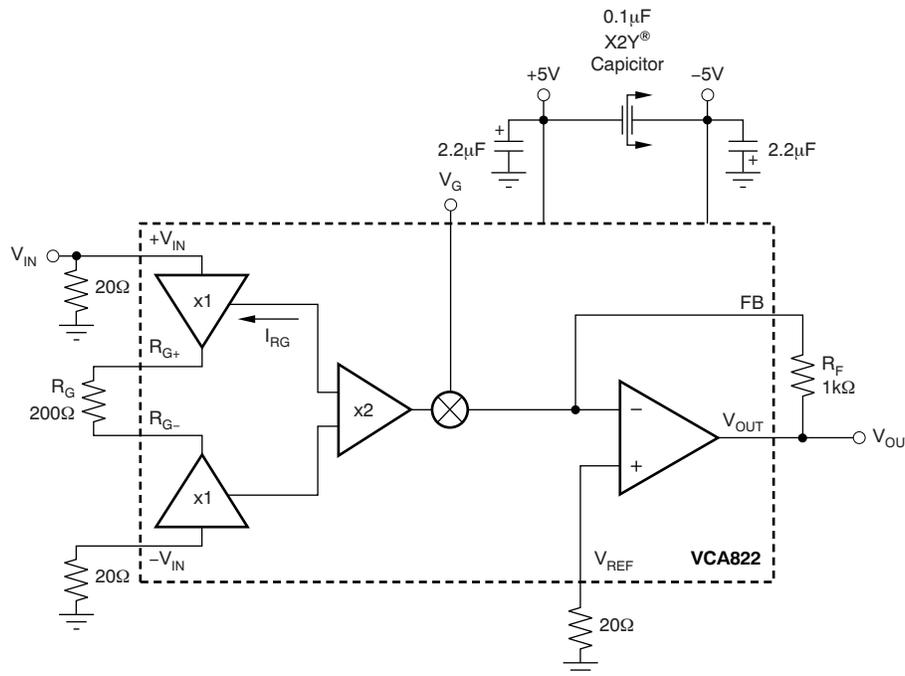
Figure 2. VCA822 Internal Schematic
