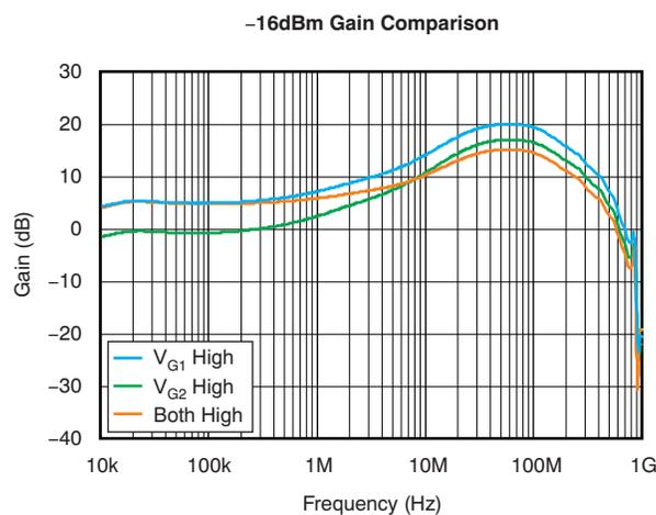
**Figure 5. Frequency Response of the Circuit for Various Gain Voltage Combinations**
