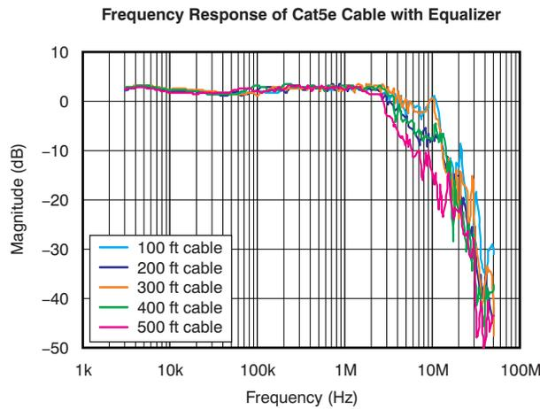
**Figure 8. Equalized AC Responses for Different Lengths of Cat5e Cable**
