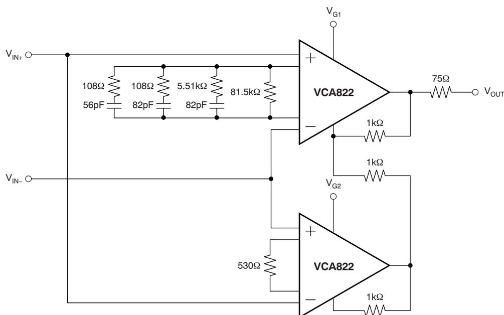
**Figure 3. Equalizer Circuit Using the VCA822**
