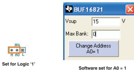
**Figure 6. BUF16821EVM Jumper JP1 Set for Logic '1'**
