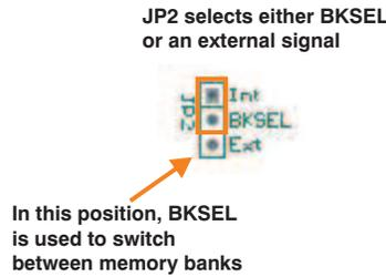
**Figure 8. BUF16821EVM Jumper JP2 Set for BKSEL Switching**
