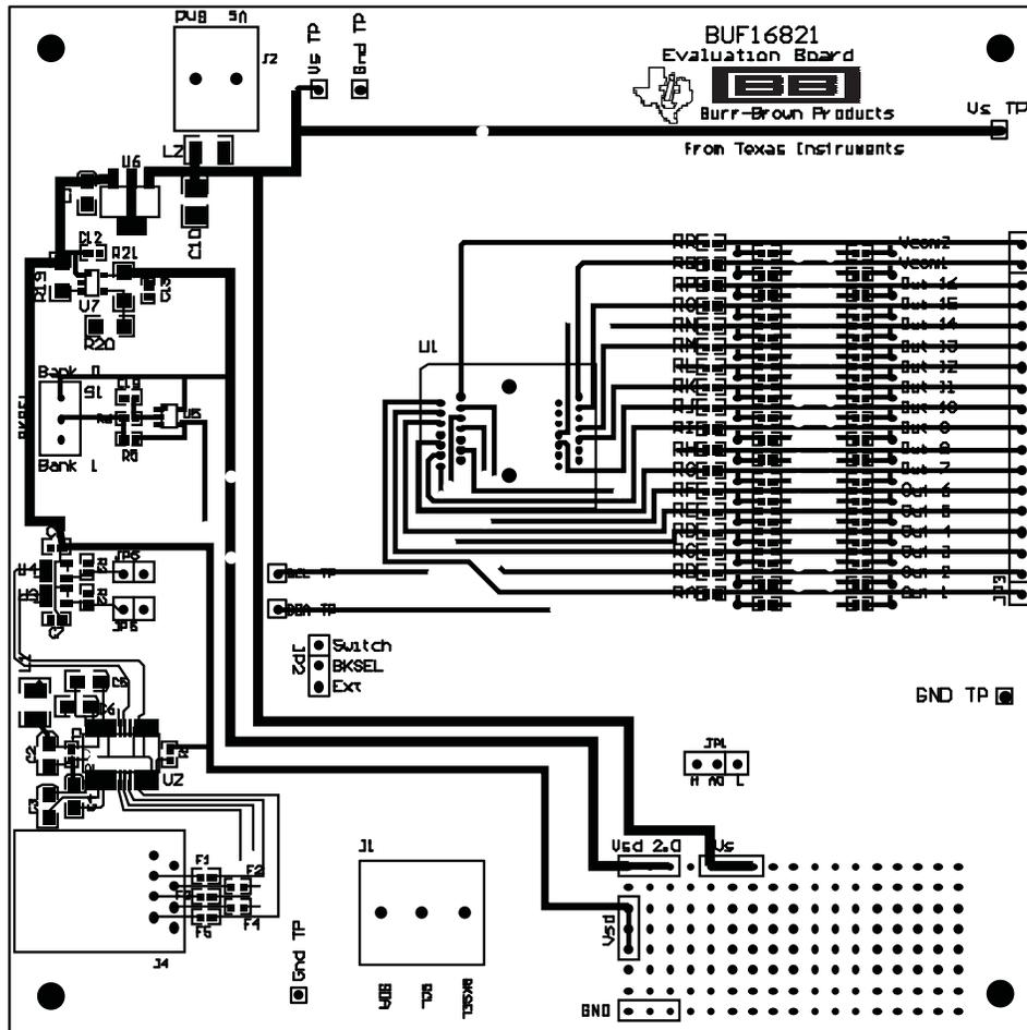
Figure 23. BUF16821EVM PCB Top Layer (Component Side)
