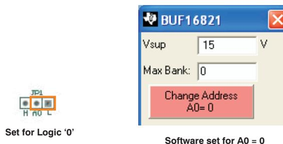
**Figure 7. BUF16821EVM Jumper JP1 Set for Logic '0'**
