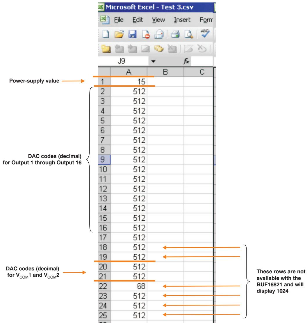
**Figure 14. Working with a Saved BUF16821 Data File**
