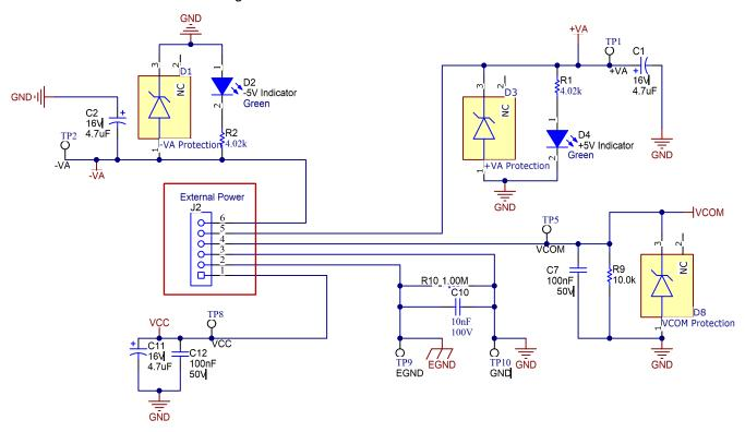
Figure 4-1. Power Terminal Block J2 Schematic
