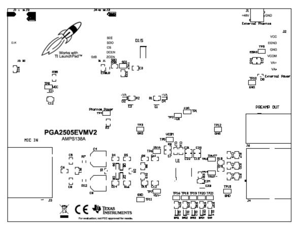
Figure 6-2. PGA2505EVMV2 Top Overlay
