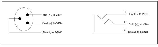
Figure 4-2. Microphone Input Connector Configuration
