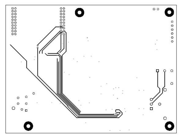
Figure 6-4. PGA2505EVMV2 Bottom Layer
