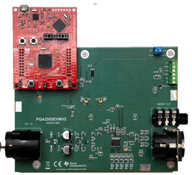
Figure 3-1. PGA2505EVMV2 With MSP430™ Microcontroller Connected
