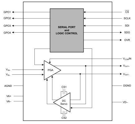
Figure 1-1. PGA2505 Functional Block Diagram
