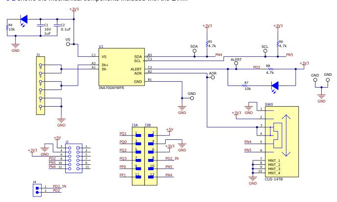
Figure 5-1. SENS113 Schematic
