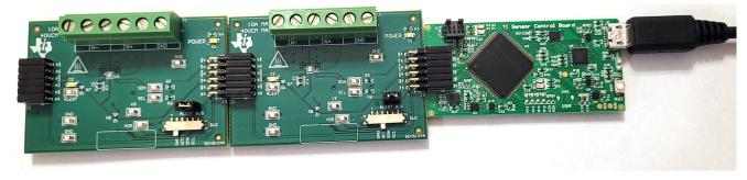
Figure 3-2. Multiple EVMs Connected to SCB Controller
