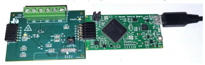
Figure 3-1. EVM (Left) Connected to SCB Controller (Right)
