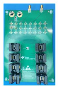
Figure 3-3. SN54SC6T07-SEP Evaluation Board (Top View)
