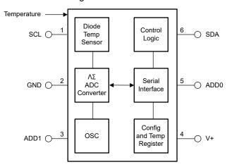
Figure 1-1. Functional Block Diagram
