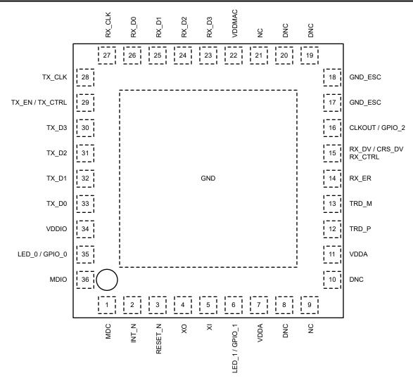
Figure 4-2. DP83TC814R-Q1 RHA Package 36-Pin VQFN
