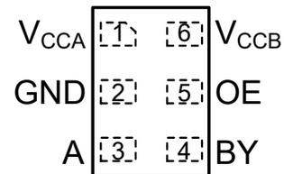
**Figure 4-2. Pin Diagram (SON) Package**
