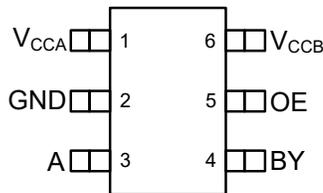
**Figure 4-1. Pin Diagram (SC70) Package**
