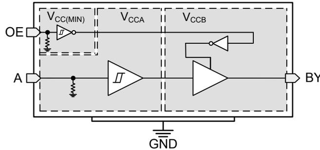
**Figure 1-1. Functional Block Diagram**
