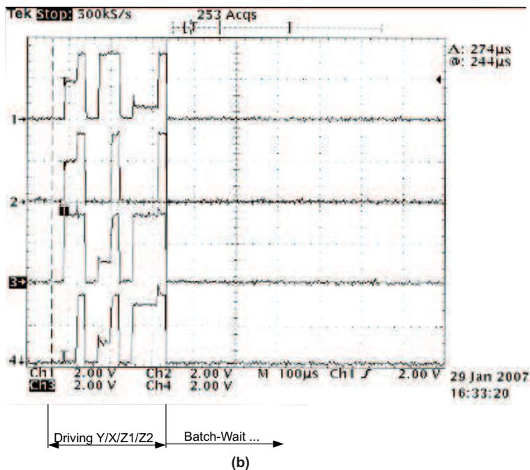
NOTE: a) Touch screen controller keeps driving, sampling, and converting X, Y, Z1, and Z2 data at a rate of  $1/(274 \mu\text{s}) = 3650$  sets per second without Batch Delay. b) The rate is controllable and the analog interface traffic is greatly reduced with Batch Delay. Where Ch1 is X+, Ch2 is X-, Ch3 is Y+, and Ch4 is Y-.
