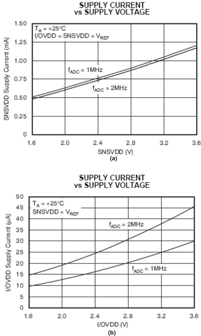
**Figure 2. Power Supply Current With Different Power Supply Voltage for (a) Analog and (b) Digital Circuitries**
