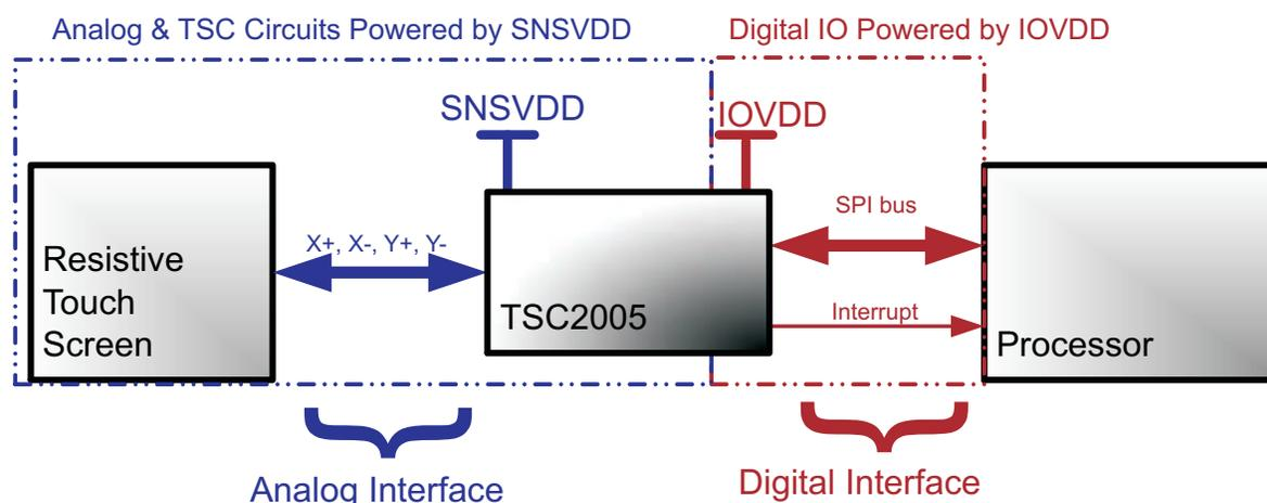
NOTE: The supply voltage on IOVDD must be the same as or lower than SNSVDD.
