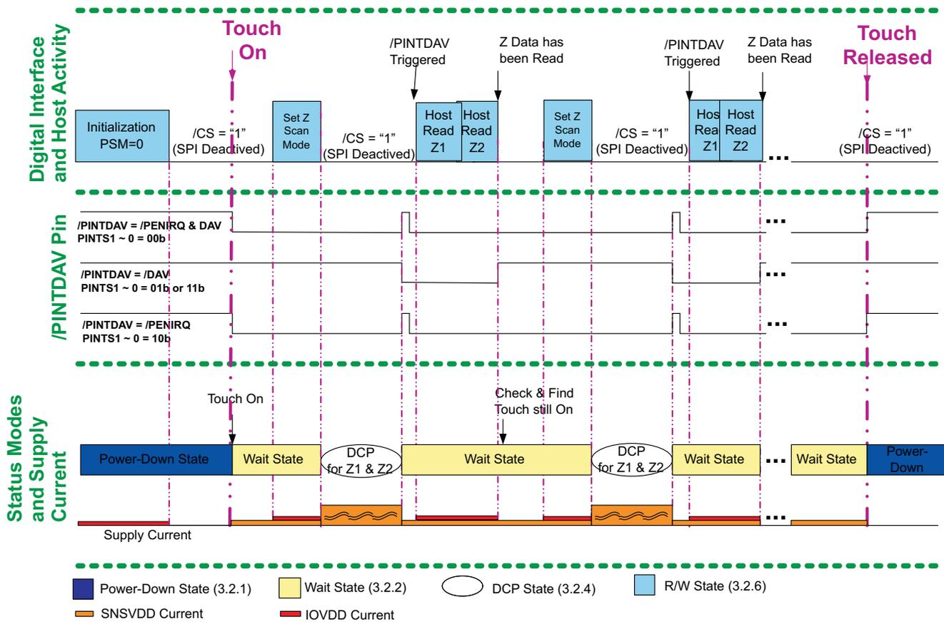
Figure 14. TSMODE3 With Z1/Z2 Converting
