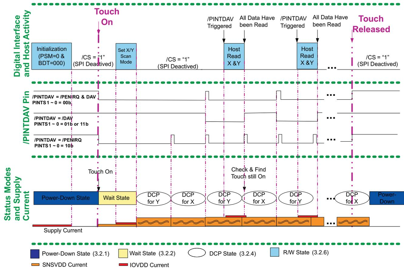
Figure 11. TSMODE2 With X/Y Converting Without Batch Delay
