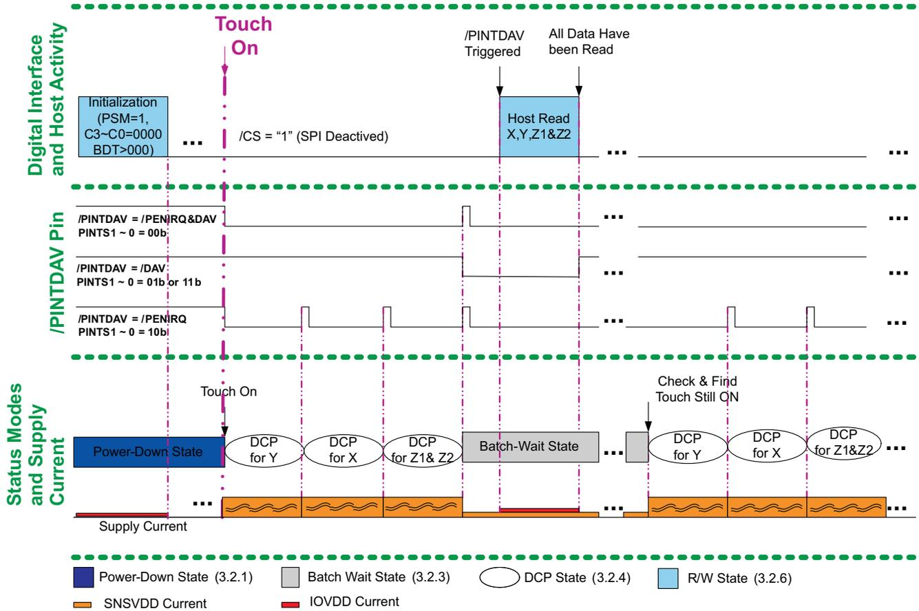
Figure 9. TSMODE1 With X/Y/Z1/Z2 Converting and With Batch Delay
