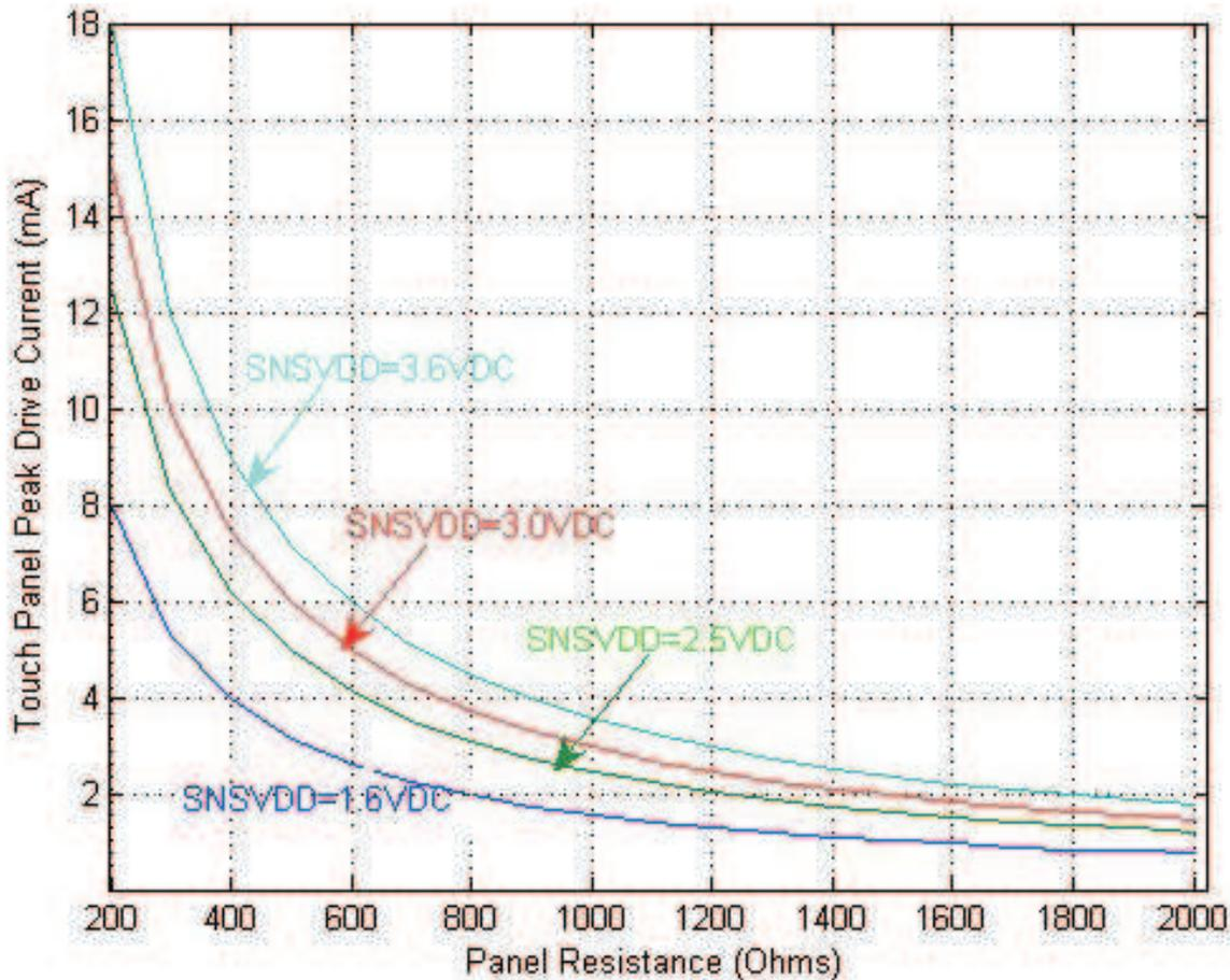
NOTE: The touch screen is driven by the touch screen controller; the panel resistance  $R_{\text{touch}}$  determines the peak drive current from the touch screen controller from the SNSVDD power supply.
