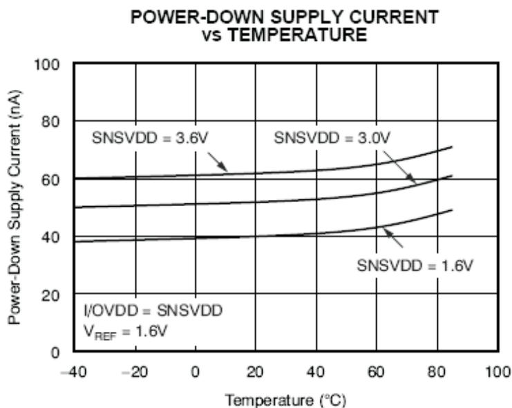
**Figure 3. Power Supply Current Under Power-Down State**
