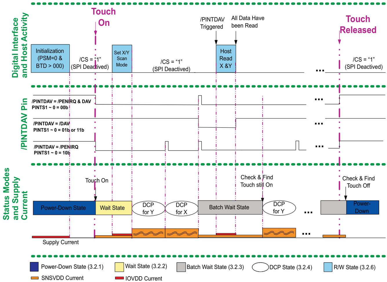
**Figure 12. TSMODE2 With X/Y Converting With Batch Delay**
