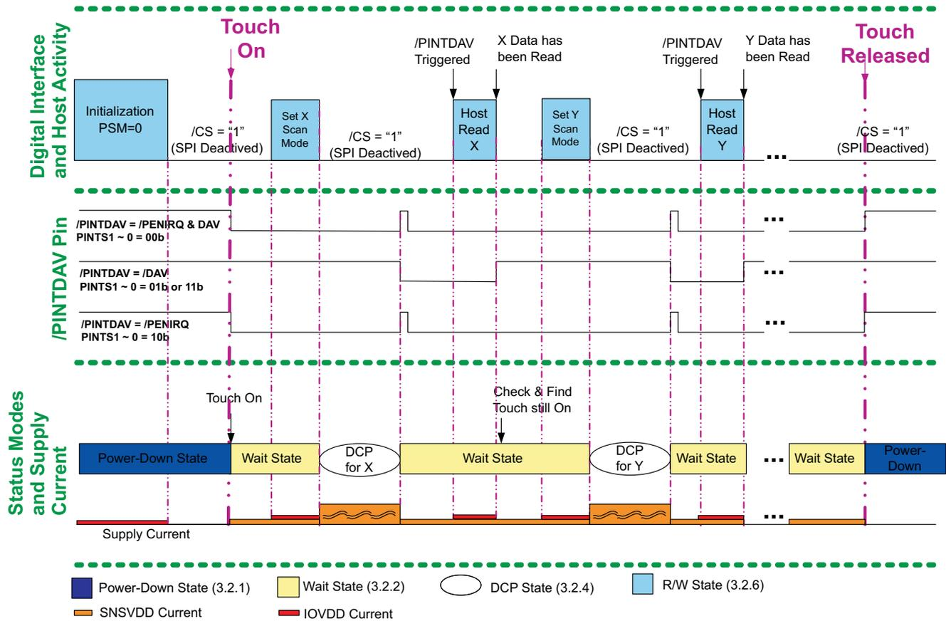
Figure 13. TSMODE3 With X/Y Converting
