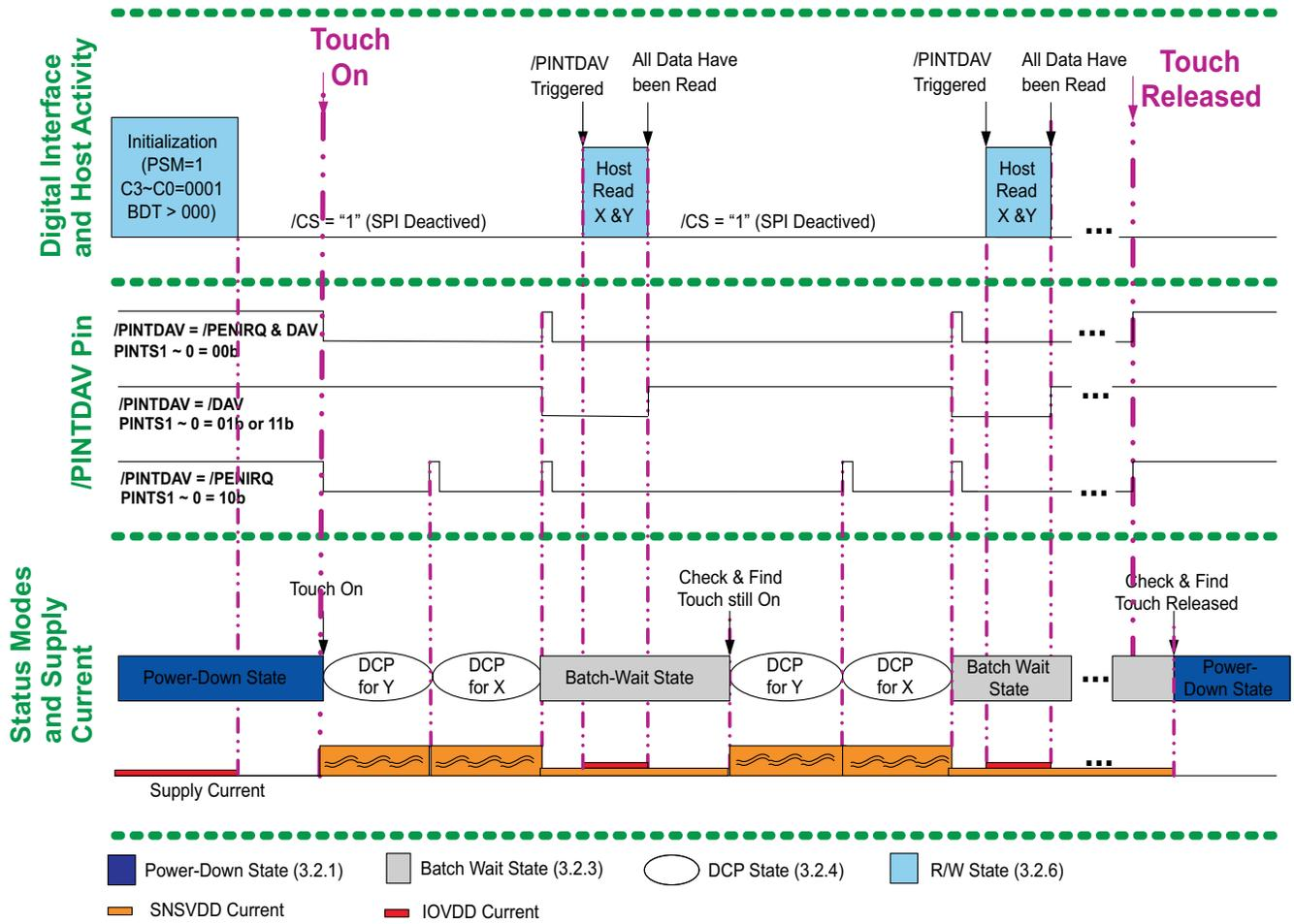
Figure 10. TSMODE1 With X/Y Converting and With Batch Delay
