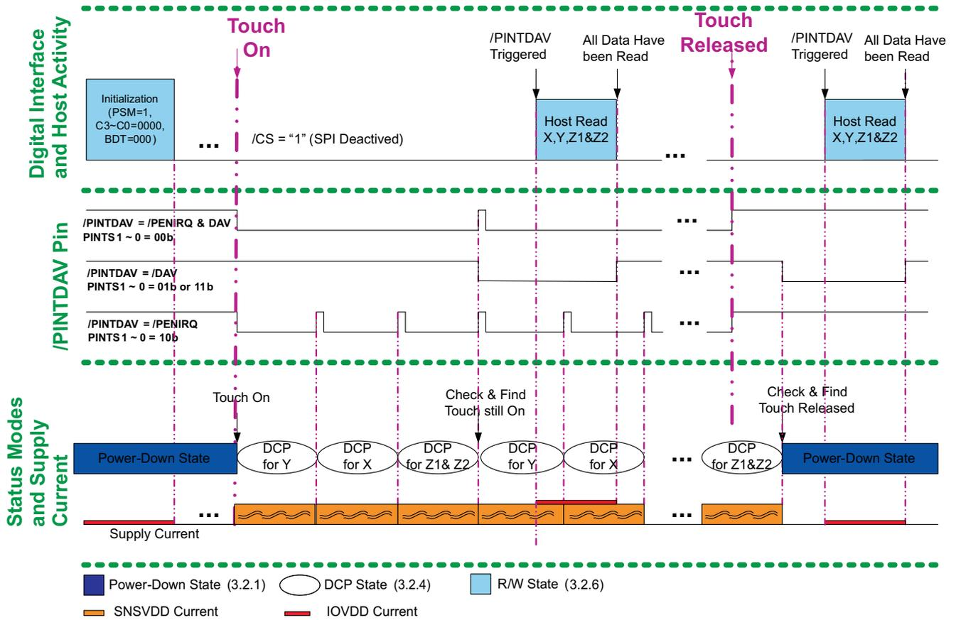
Figure 8. TSMODE1 With X/Y/Z1/Z2 Converting and Without Batch Delay
