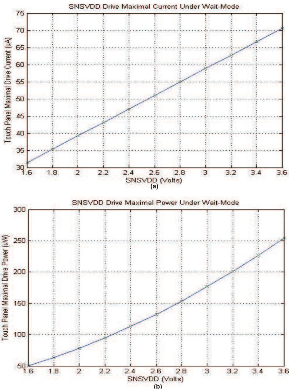
**Figure 5. Power Supply SNSVDD Maximal (a) Current and (b) Power in Wait State**
