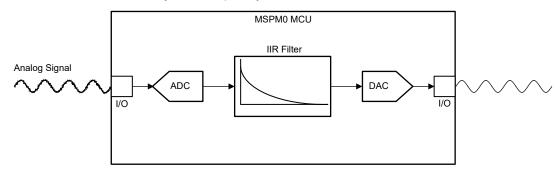
Figure 1-1. IIR Filter Functional Block Diagram
