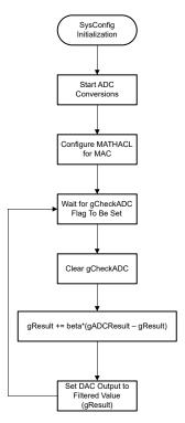
Figure 6-1. Example Software Sequence
