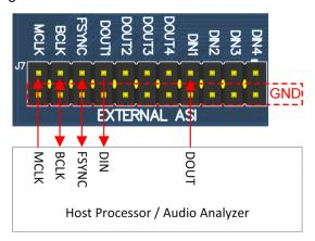
Figure 2-6. AC-MB Connection with External Audio Serial Interface
