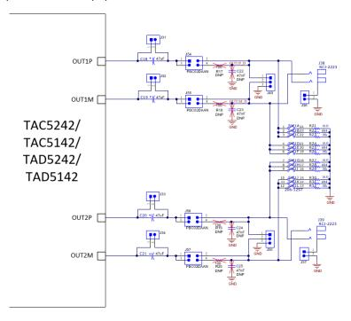
Figure 2-9. TAC5242/TAC5142/TAD5242/TAD5142 EVM Output Architecture
