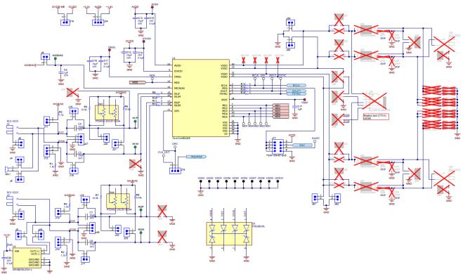
Figure 4-5. TAA5242 EVM Main DUT Schematic
