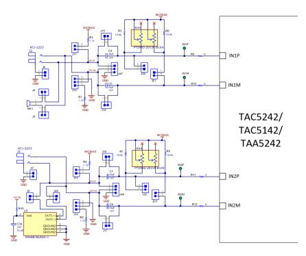
Figure 2-8. TAC5242/TAC5142/TAA5242 EVM Input Architecture for Channel 1 and 2
