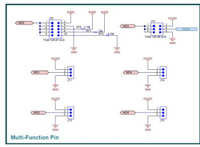
Figure 4-4. TAC5142 EVM Connectors and Supporting Circuitry Schematic
