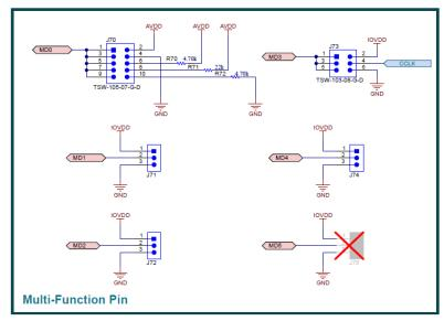
Figure 4-6. TAA5242 EVM Connectors and Supporting Circuitry Schematic
