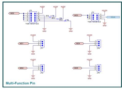
Figure 4-8. TAD5242 EVM Connectors and Supporting Circuitry Schematic
