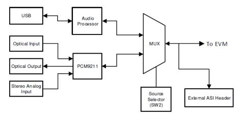
Figure 2-2. AC-MB Audio Interface Block Diagram
