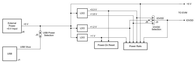
Figure 2-7. Power-Supply Distribution of the AC-MB
