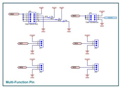
Figure 4-10. TAD5142 EVM Connectors and Supporting Circuitry Schematic
