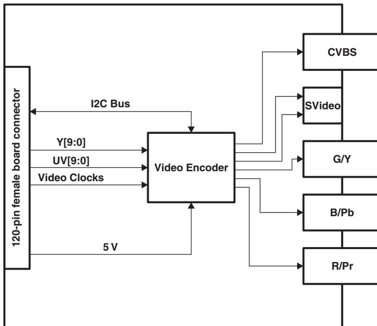
Figure 1-2. Encoder Module
