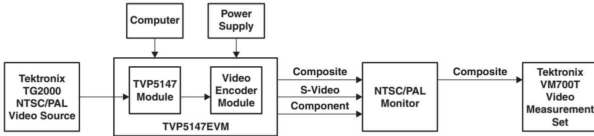
Figure 1-5. TVP5147EVM System Level Block Diagram
