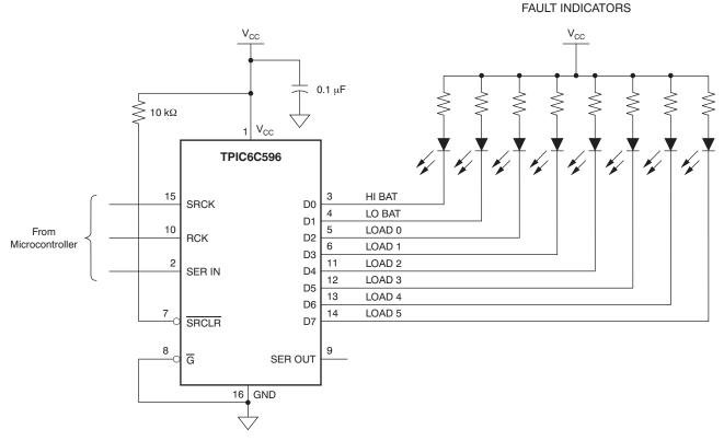
Figure 1. TPIC6C596 Used as Fault Indicator
