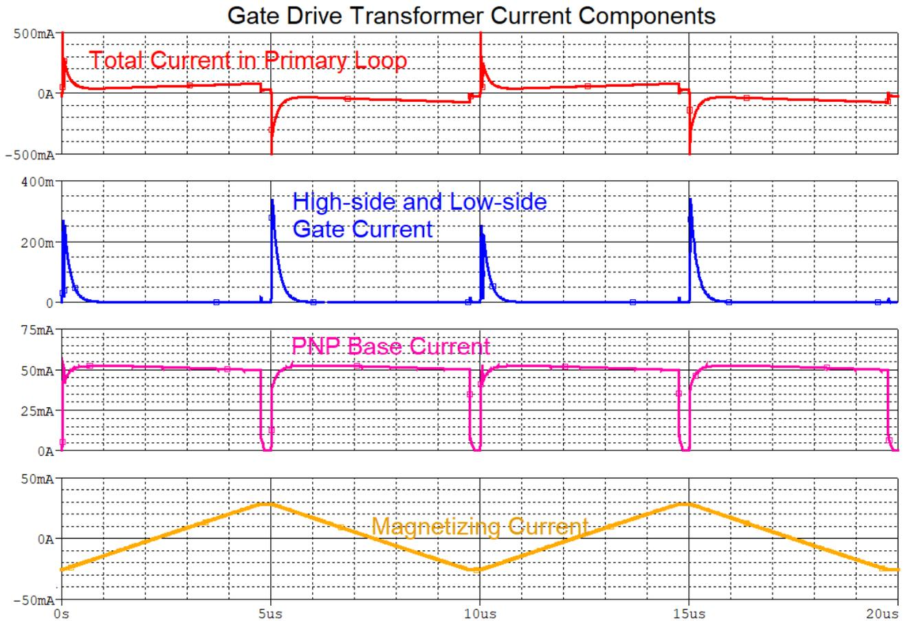
**Figure 4-1. Simulation Showing the Major Current Components in the Gate Drive Circuit**
