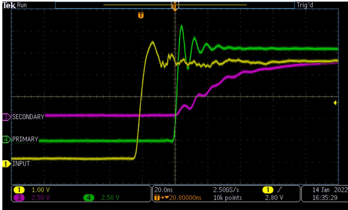
**Figure 3-1. Oscilloscope Capture Showing Propagation Delay From the Driver IC and Transformer From a Circuit**
