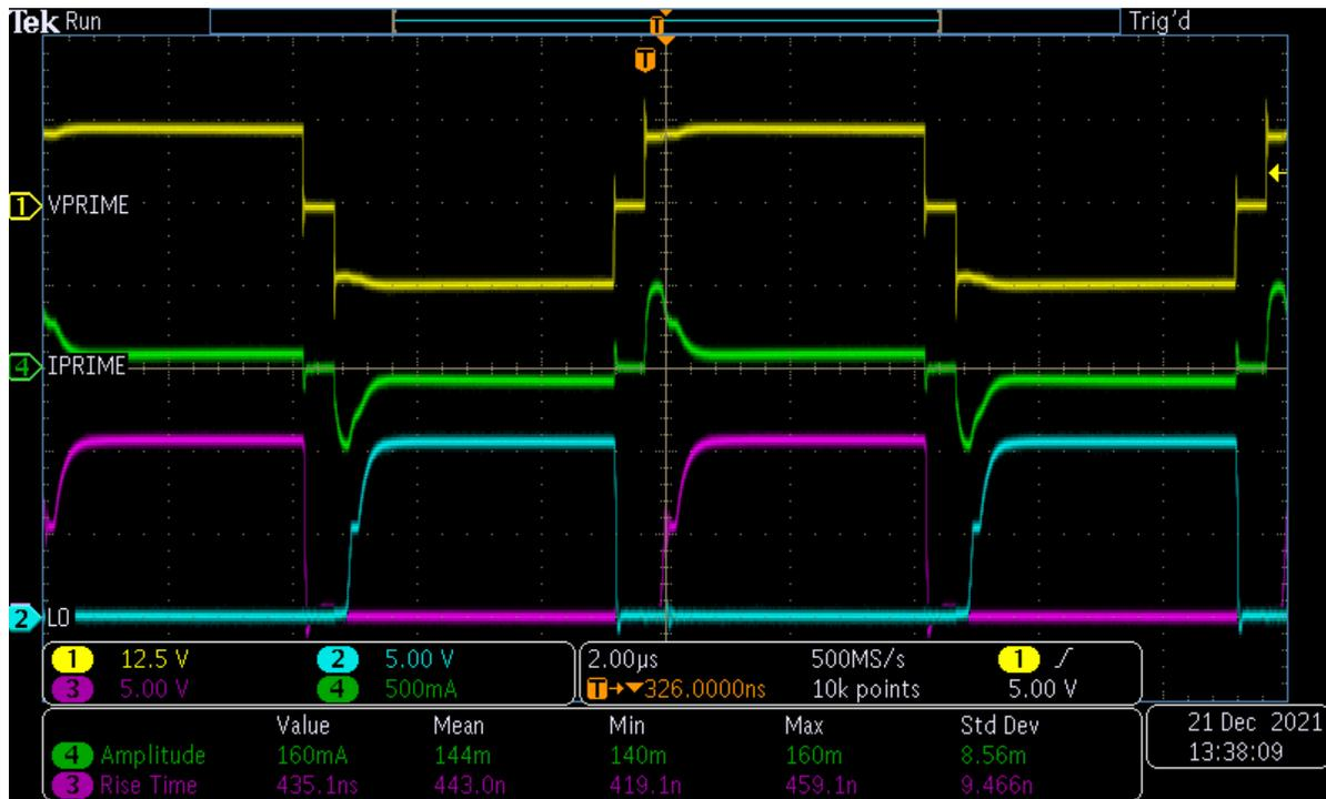
Figure 4-2. Oscilloscope Capture of Gate Drive Transformer Waveforms With 100Ω R<sub>B</sub>
