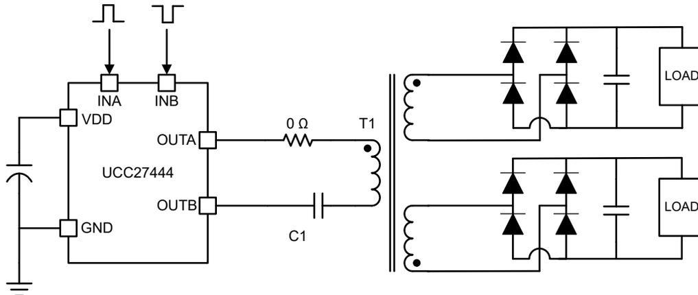
**Figure 4-3. Example Schematic of a Push-Pull Bias Supply Using the UCC27444 Gate Driver IC**
