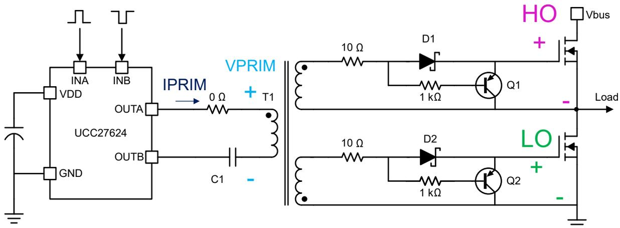
**Figure 2-3. Schematic of a Push-Pull Gate Drive Circuit With Colored Labels for Primary Current, Primary Voltage, and HO and LO**
