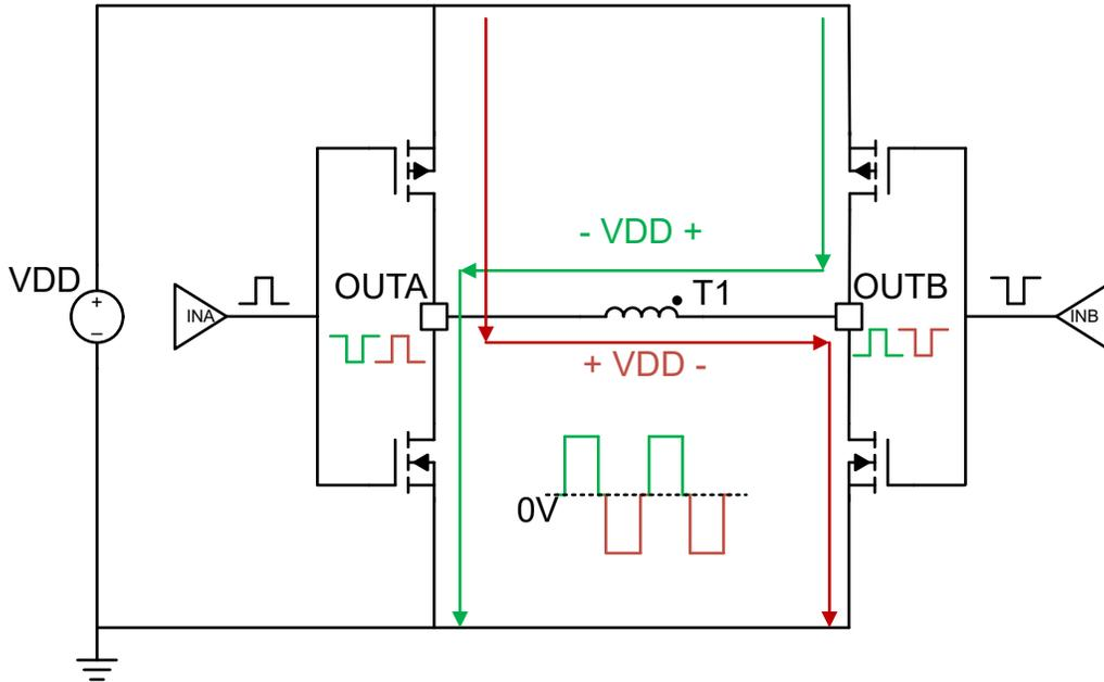
**Figure 2-2. Simplified Schematic Showing Current Flow Through the Driver Output Stage in a Push-Pull Topology**
