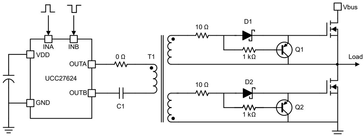
**Figure 2-1. Example Schematic of a Push-Pull Gate Drive Circuit Used to Drive a Half-Bridge**
