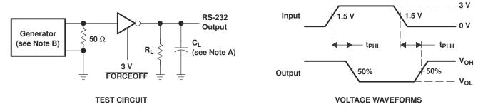
NOTES: A. C<sub>1</sub> includes probe and jig capacitance.
