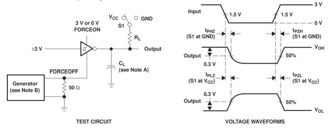
NOTES: A.  $C_L$  includes probe and jig capacitance.
