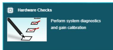
Perform a system calibration before proceeding to the *Tuning and Audio Processing* window. If an attempt to enter the *Tuning and Audio Processing* window is made before performing hardware checks, PPC3 prompts with a window requesting to perform the verification of the hardware. Only new sessions require a hardware check, so this window will not appear when continuing from a previous session or loading a previously saved one.
