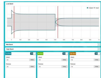
All the multiband AGL functions are also featured in the full-band AGL window. By default, -1 dB is configured for full-band AGL and the attack and release rates are set to 10 V/ms.
