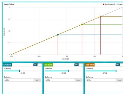
An *Input/Output* chart is available to easily configure the threshold levels for each band. Drag and select each threshold and fine tune the desired threshold level by controlling the levels in the lower part of the window. Modify the *Softening* parameter to configure the sharpness of the compression knee of the AGL.
