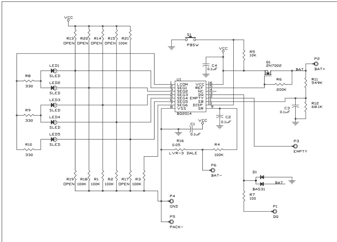
Figure 4. bq2014 Li-Ion Battery Capacity Monitoring System
