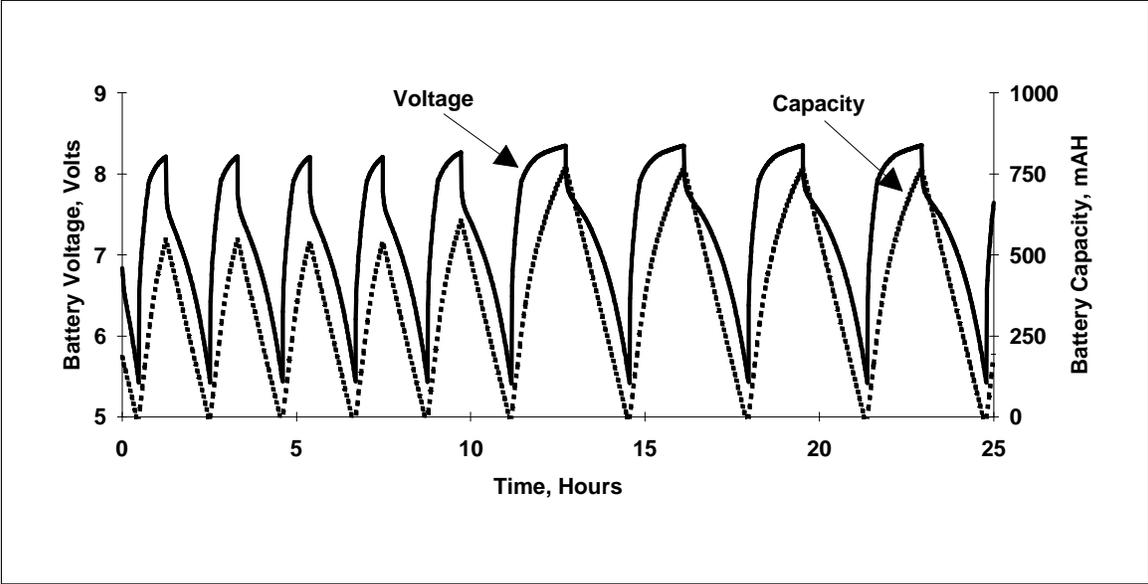
Figure 5. Li-Ion Battery Discharge and Capacity Profile
