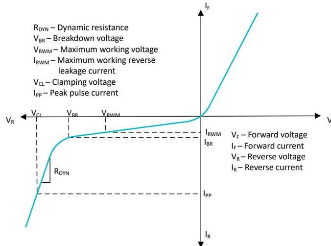
**Figure 4-1. TVS Diode Characteristics**
