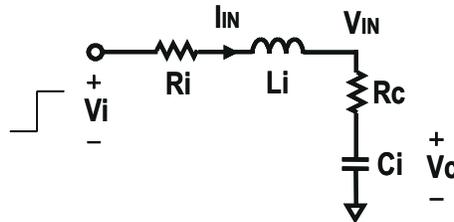
**Figure 2-1. Simplified Equivalent Circuit During Adapter Insertion**
