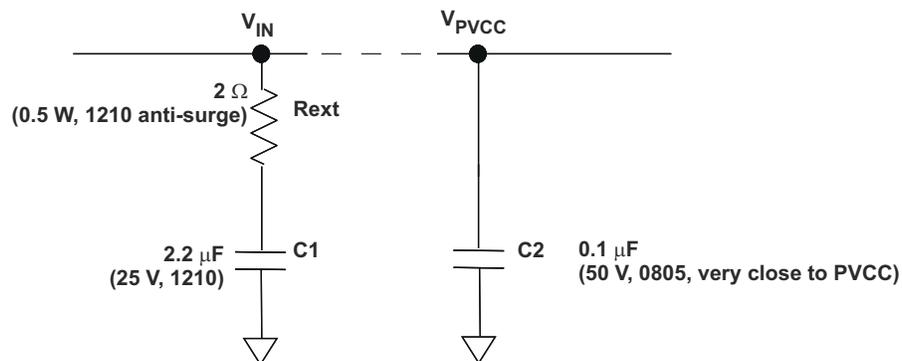
**Figure 3-1. Recommended Input Filter Design**
