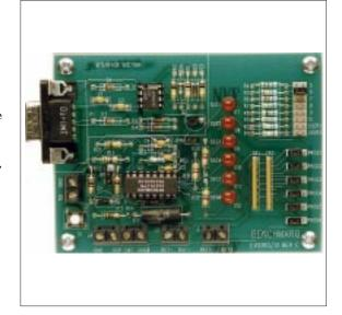
The menu-driven software provided with the EV2010 displays charge/discharge activity and allows user interface to the bq2010 from any standard DOS PC.
