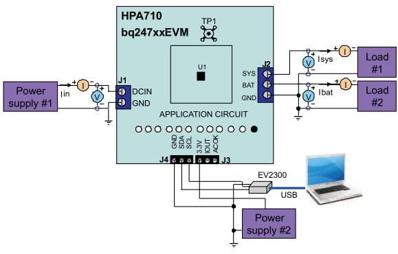
Figure 4. Test Setup for HPA710
