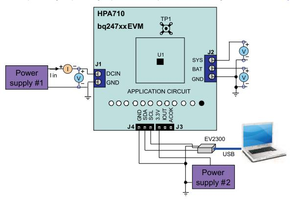
Figure 2. Original Test Setup for HPA710
